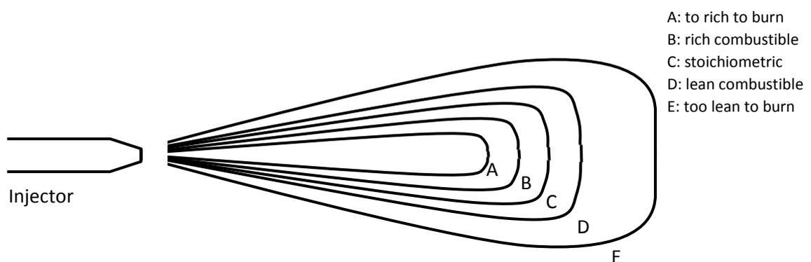
Fig.1-8 Schematic of fuel jet of diesel spray, showing air-fuel vapor zones around the inner liquid core.
