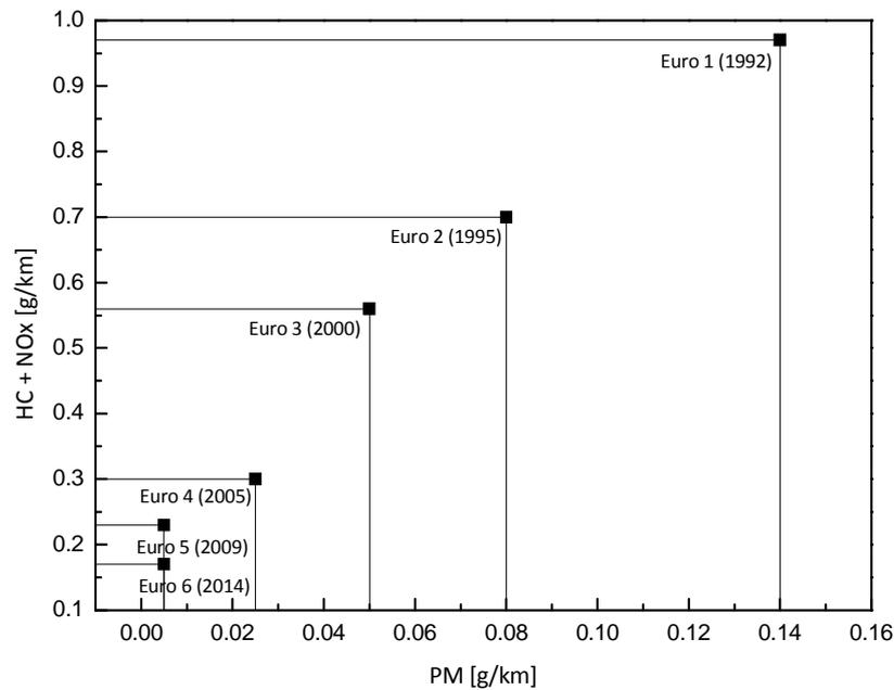
Fig.1-2 Progression of European air emission standard for diesel car[3]
