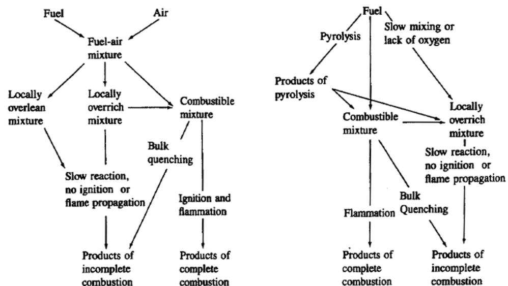
Fig.1-5 Schematic representation of diesel hydrocarbon formation mechanisms[12]
