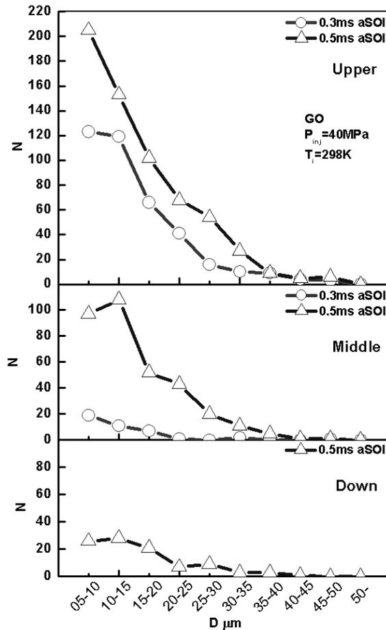
Fig.7-9 Droplet distribution of gas oil ( $P_{inj}=40MPa$ ,  $T_i=298K$ )
