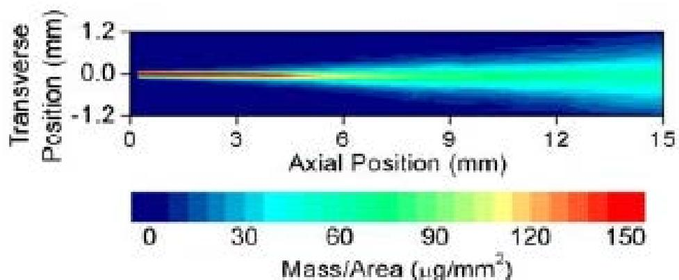
Fig.2-2 Example of spray mass/area distribution result by using x-ray measurement technique (750  $\mu$ s aSOI,  $P_{inj}$ =1000 bar,  $P_{amb}$ =30 bar) [16]
