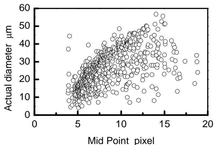
Fig.3-8 Correlation between Mid Point and actual diameter of particles
