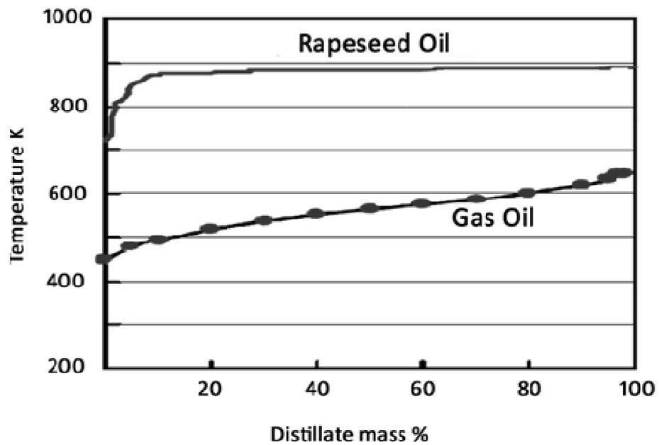
Fig.2-13 Distillation characteristics of test fuel
