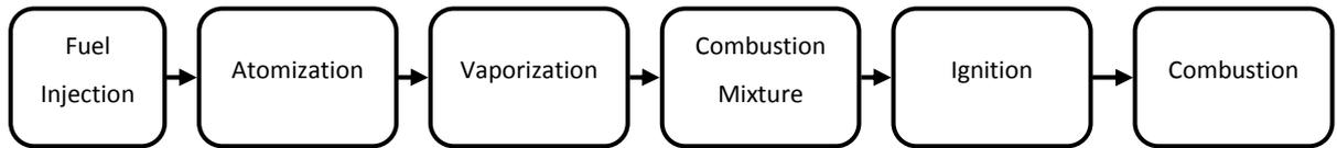
Fig.1-7 Events after fuel injection leading to combustion in diesel engine
