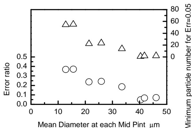
Fig.3-12 Relation between accuracy of particle diameter measurement and particle diameter
