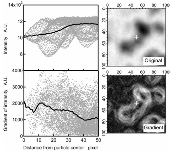
Fig.3-5 Gradient intensity profile on irregular shape of droplets
