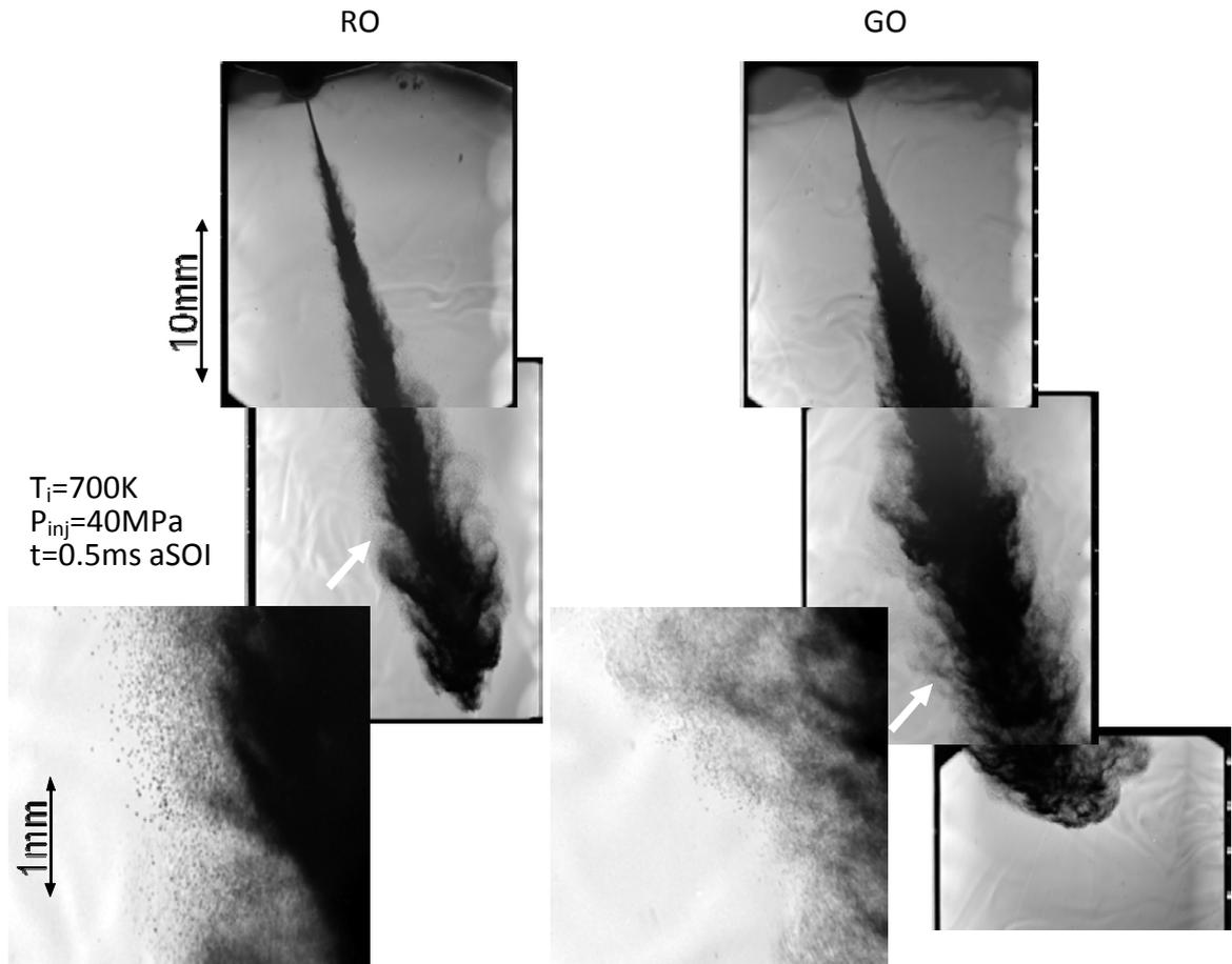
Fig.4-3 Comparison of spray structure and droplets between rape-seed oil and gas oil sprays ( $T_i=700K$ ,  $P_{inj}=40MPa$ )
