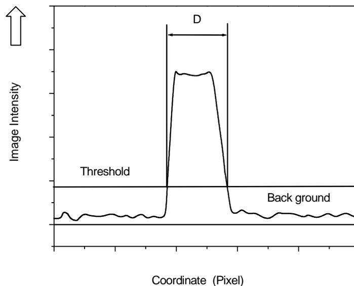
Fig.3-1 Thresholding level effect on a droplet size
