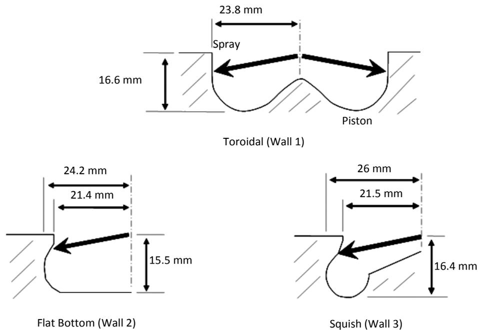
Fig.6-1 Geometry of impinging wall
