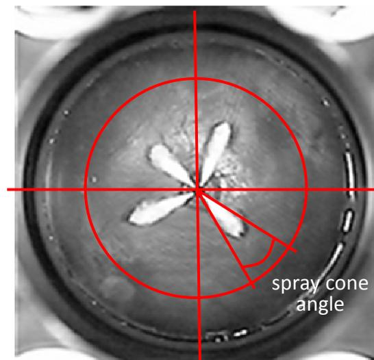
Fig.5-2 Spray cone angle analysis example. Measurement were made for each hole spray jet
