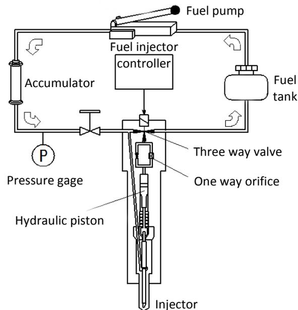
Fig.2-8 High pressure fuel injection system
