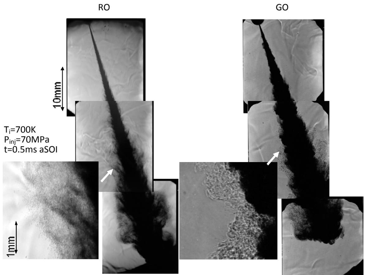
Fig.4-4 Comparison of spray structure and droplets between rape-seed oil and gas oil sprays (T<sub>i</sub>=700K, P<sub>inj</sub>=70MPa)
