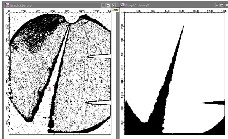
Fig.3-17 Liquid phase binary image extracted from the initial binary image
