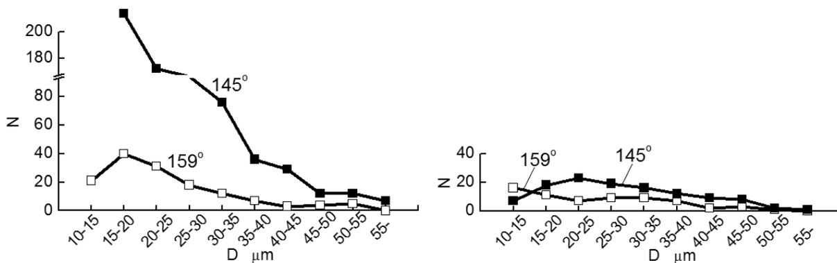
Fig.6-7 Droplet distribution comparison of spray nozzle angle (Toroidal,  $P_{inj}=40\text{MPa}$   $T_i=298\text{K}$ , 0.5ms aSOI)
