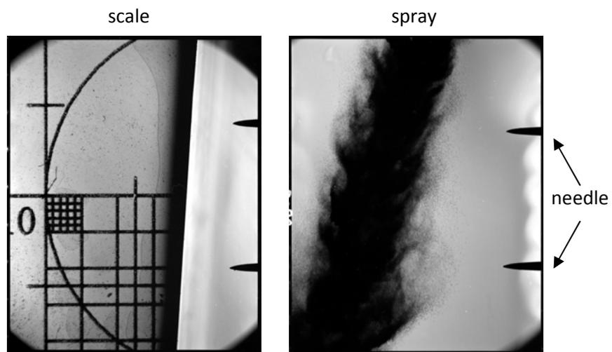
Fig.3-13 Example of spray and scale with reference needle
