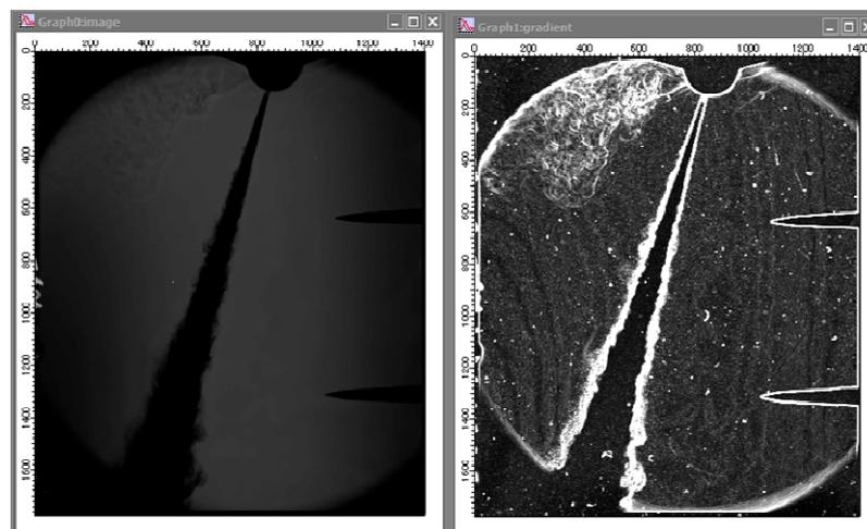
Fig.3-16 Gradient image produced from original TIFF image
