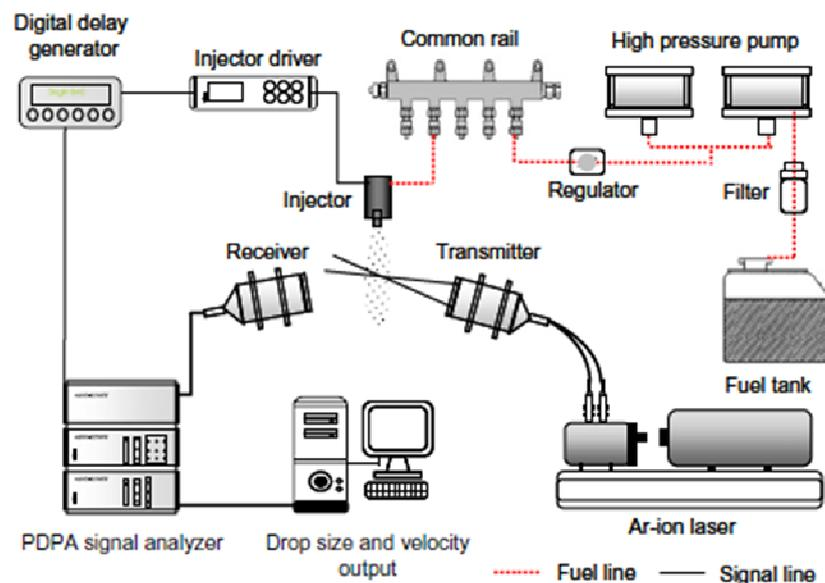
Fig.2-1 Droplet particle analyzer system using PDPA [15]
