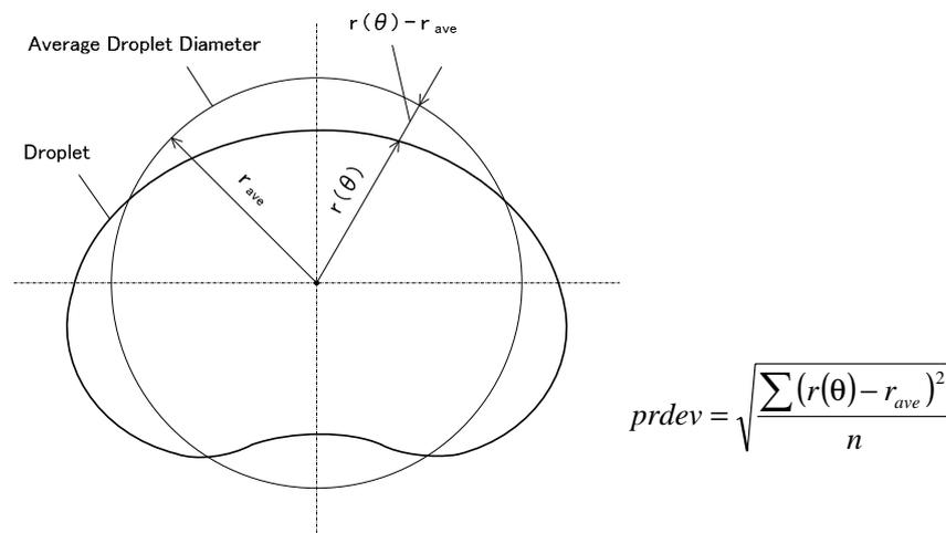
Fig.3-6 Schematic deviation of particle radius
