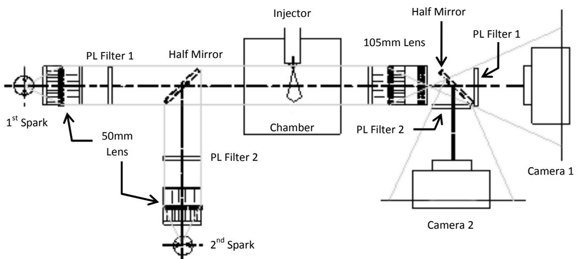
Fig.2-17 Optical setting for dual nano-spark shadowgraph photography method
