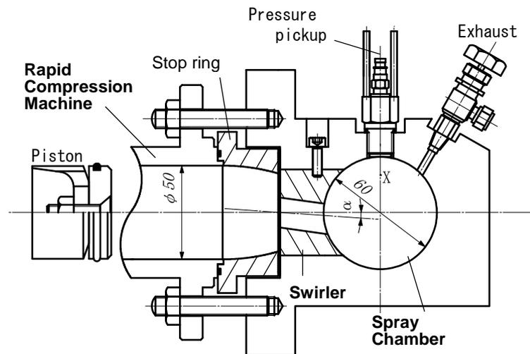
Fig.7-1 Chamber cross section with swirler
