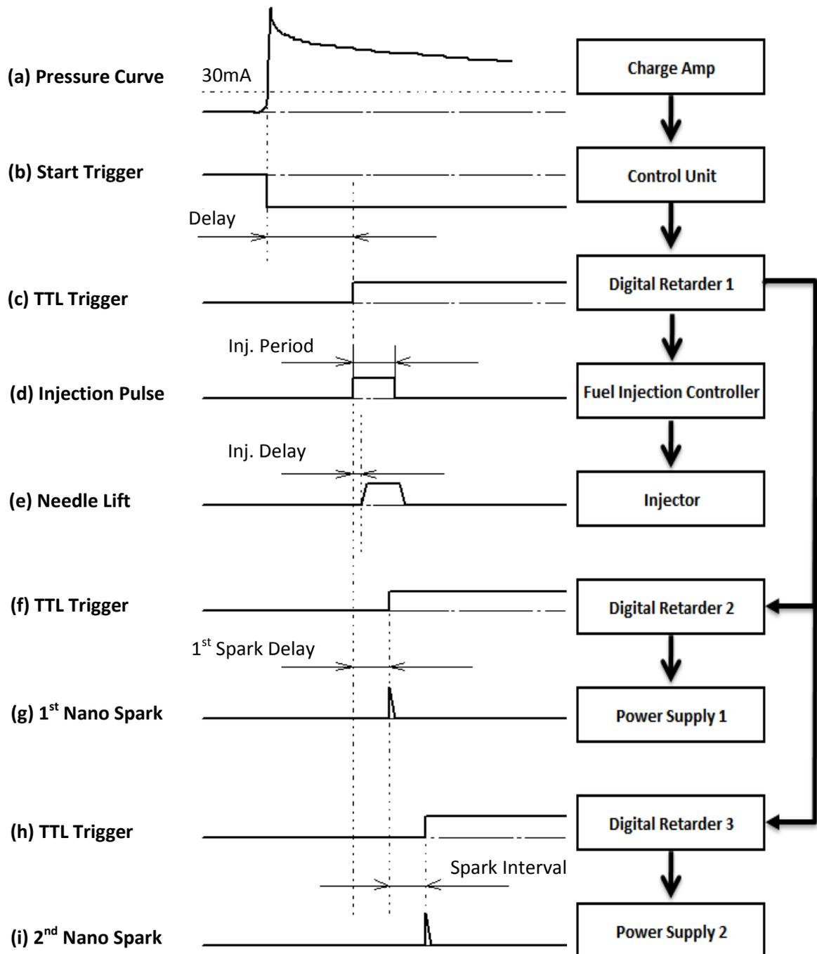
Fig.2-11 Electronic circuit pulse sequence during nano-spark photography
