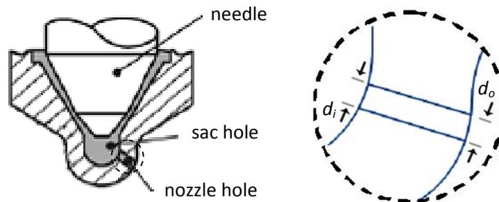
Fig.5-1 Schematic diagram for direct injection diesel engine spray nozzle
