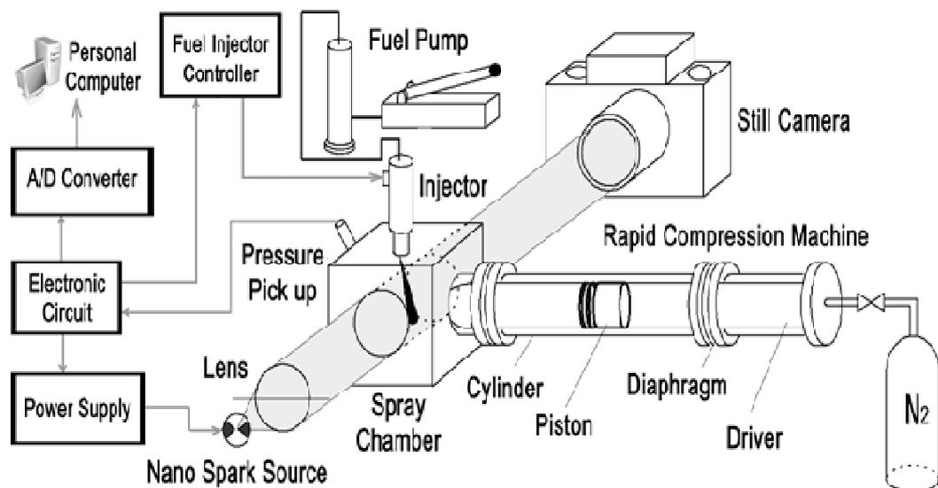
Fig.2-5 Schematic diagram of nano spark shadowgraphy method
