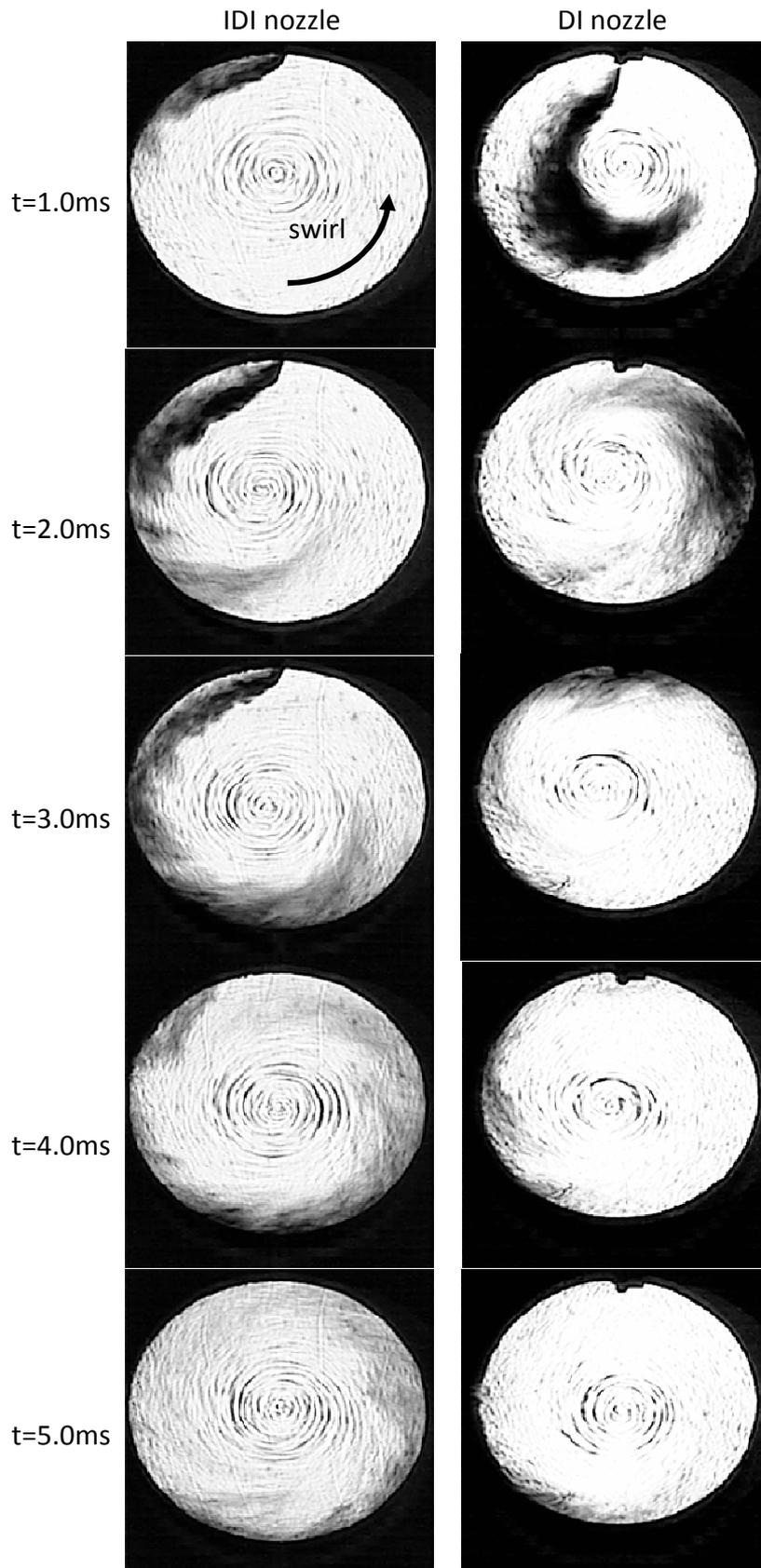
Fig.7-10 Comparison between IDI nozzle and DI nozzle rapeseed oil spray development under swirl influence ( $P_{inj}=40\text{MPa}$ ,  $T_i=700\text{K}$ )
