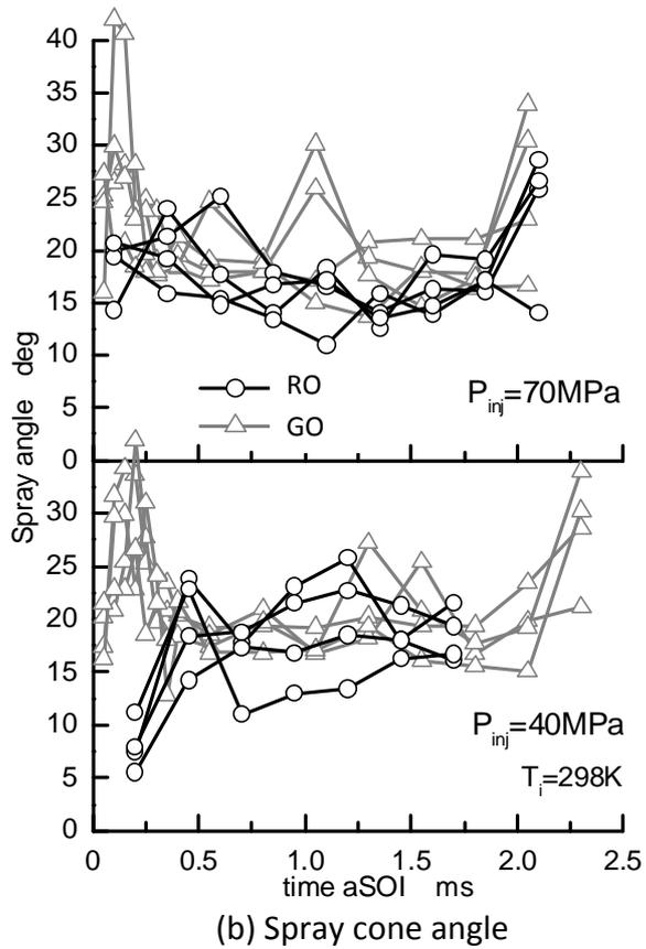
Fig.5-4 Variation of spray penetration and cone angle
