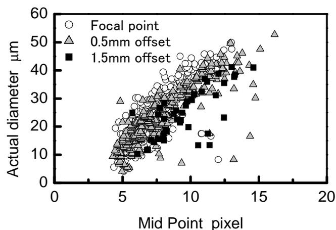
Fig.3-11 Effect of deviation from focal depth on correlation Mid Point and particles actual diameter
