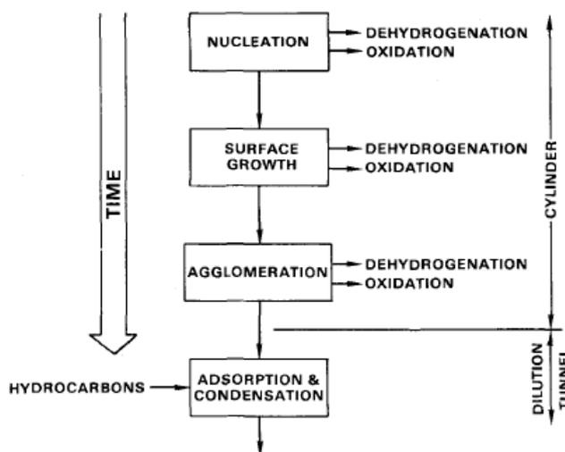
Fig.1-4 Processes to leading of net production of diesel particulates[10]
