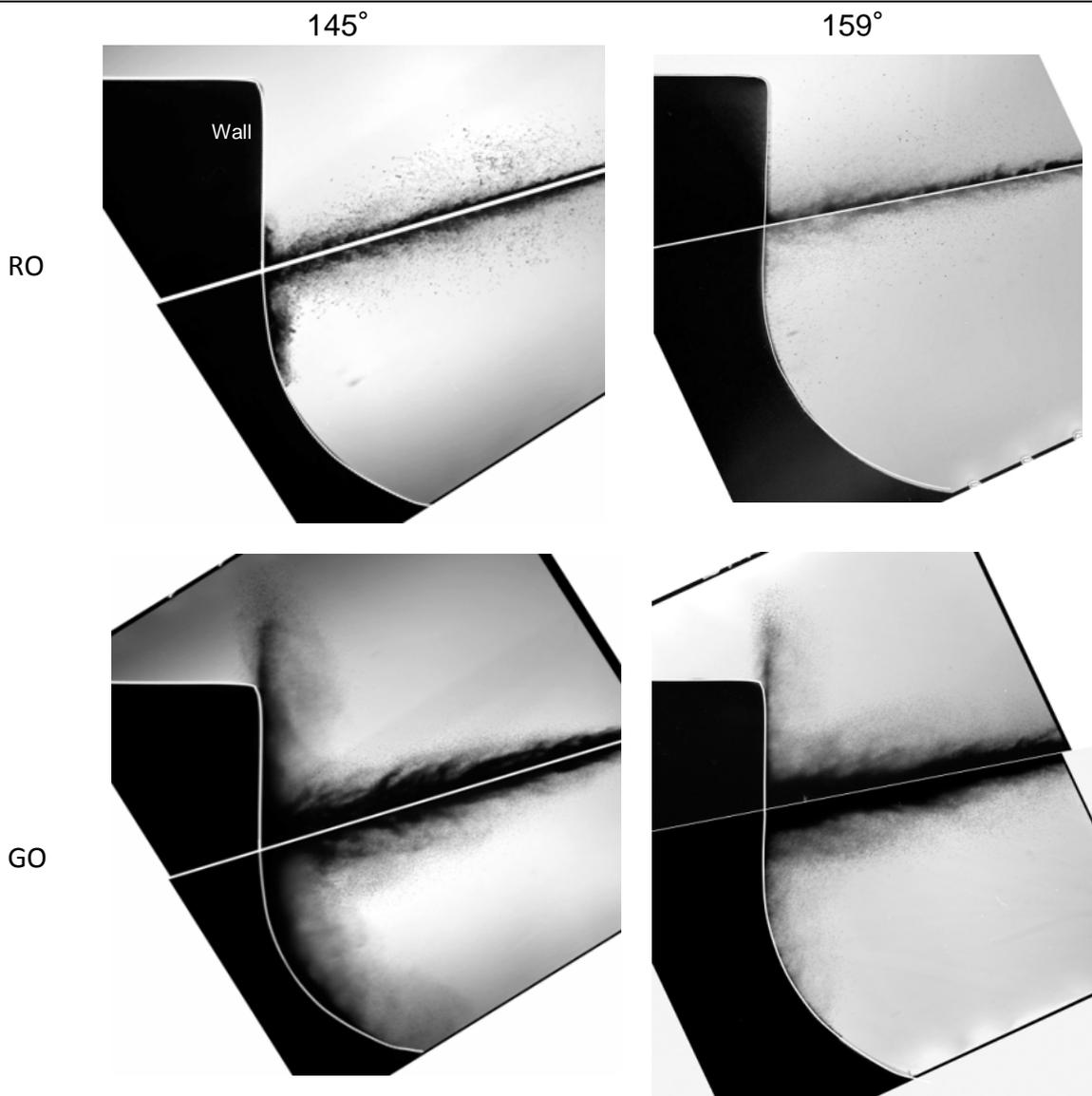
Fig.6-6 Comparison on the effect of spray nozzle angle to wall impingement ( $P_{inj}=40\text{MPa}$   $T_i=298\text{K}$ , 0.5ms aSOI)
