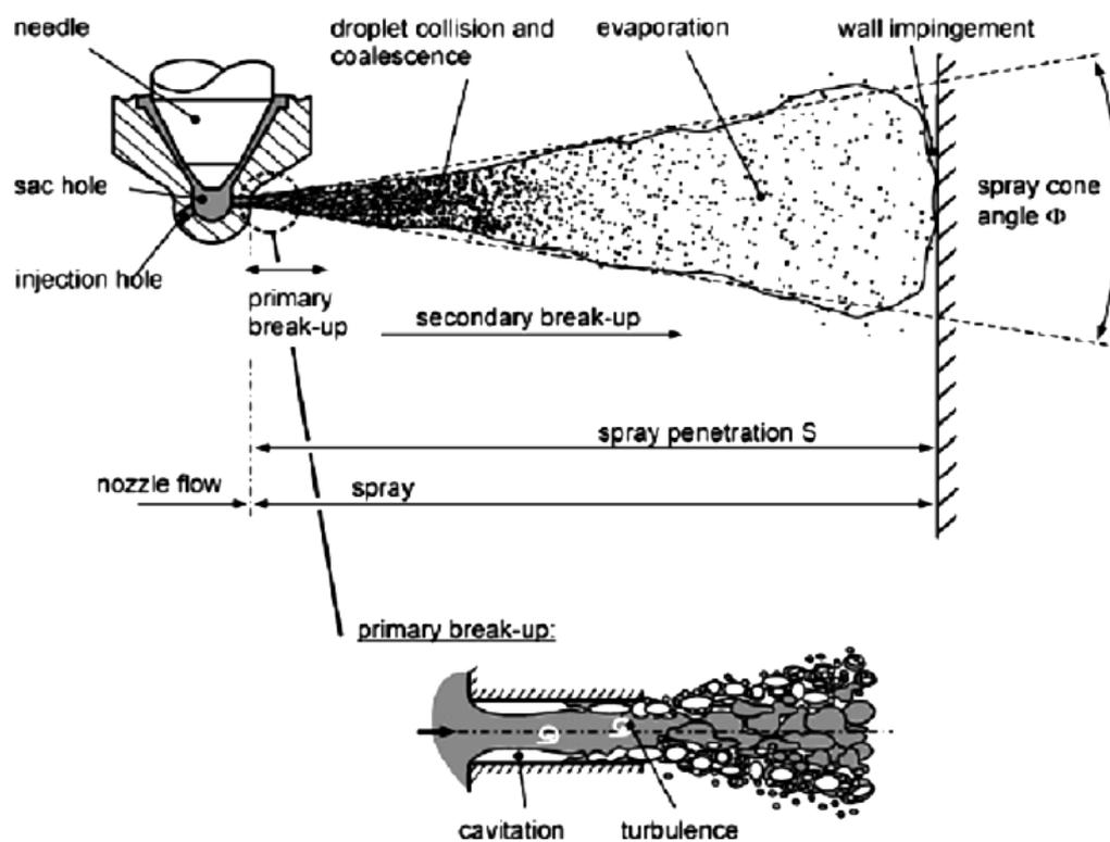
Fig.1-6 Schematic of full cone spray[39]
