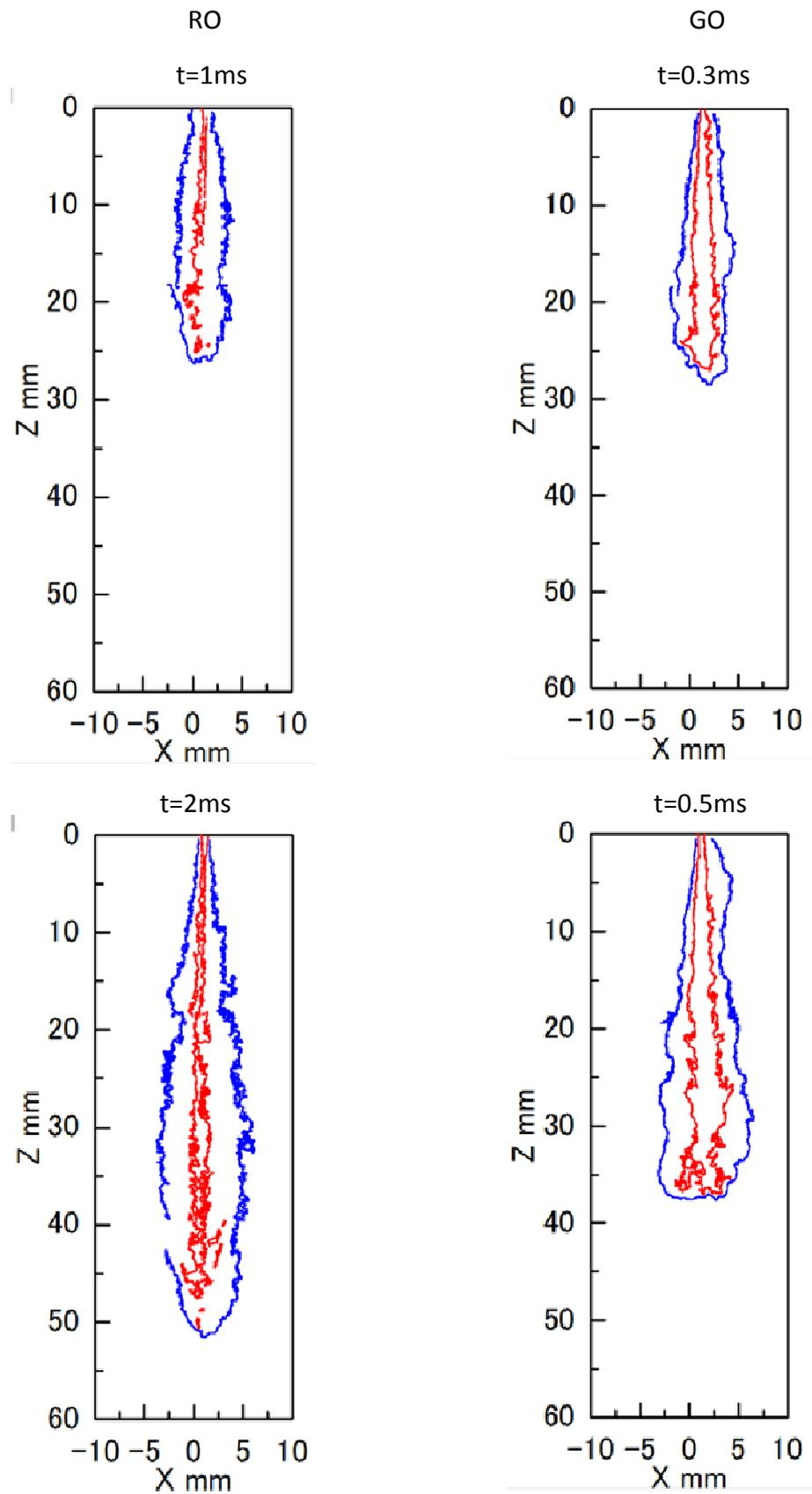
Fig.7-6 Spray development outline and progression of liquid core in IDI nozzle ( $P_{inj}=40\text{MPa}$ ,  $T_i=700\text{K}$ )
