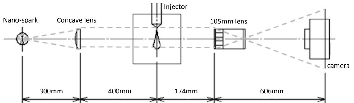
Fig.2-15 Optical setting for single spark shadowgraph method
