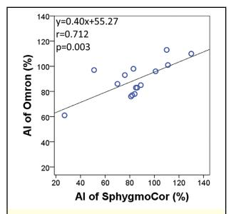
**Figure 2.** Relationship between augmentation index (AI) in the radial artery determined using the SphygmoCor device and that measured using the HEM-9000AI (Omron) device.
