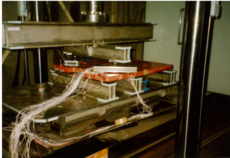
Fig. 3.6 Test condition of the static load
