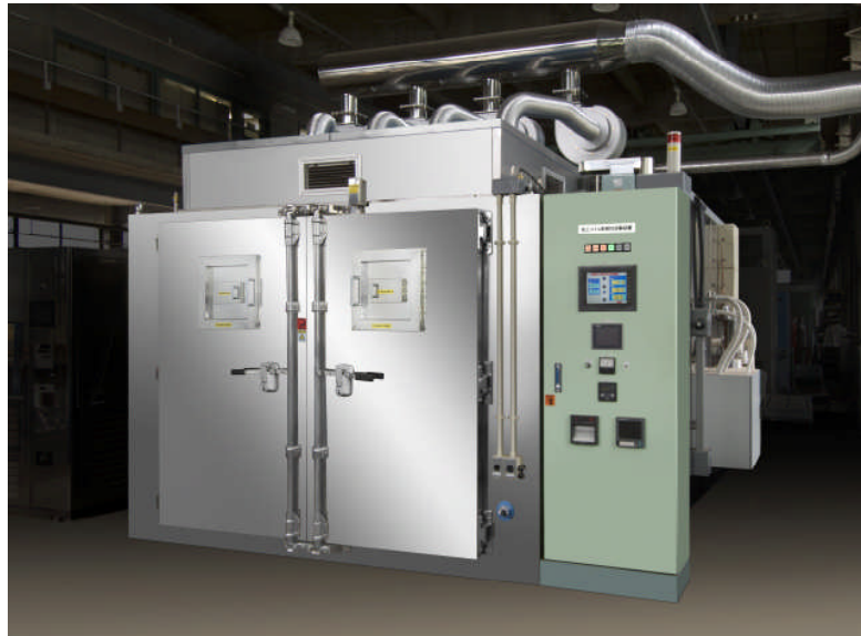
Fig. 5.24 Appearance of ultra-accelerated weathering test equipment for ground coil
