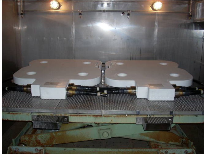
Fig. 5.26 Accelerated weathering test situation of PLG coil
