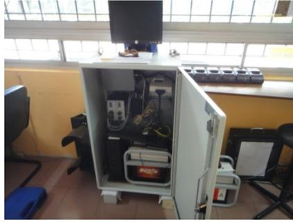
Figure 3.1(b) The CPU of the WIM system
