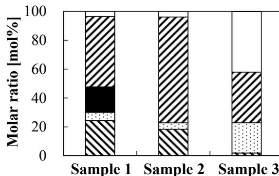
**Fig. 4** Molar ratios of each element contained in the various samples; Sample 1, slag solution; Sample 2, the Fe-free solution; Sample 3, precipitated sample. Bars:  $\square$ ,  $\text{///}$ ,  $\blacksquare$ ,  $\text{□}$ , and  $\text{▨}$  were P, Ca, Fe, Mn,
