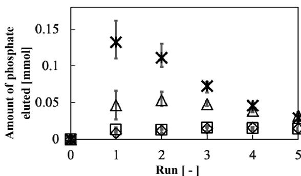
**Fig. 2** Elution behavior of phosphate from the dephosphorization slag using various concentrations of HNO<sub>3</sub>. Symbols: \*, Δ, ◇, and □ = 0.5, 0.2, 0.1, and 0.05 mol/L HNO<sub>3</sub> as an eluate
