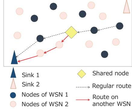
Fig. 3. Example of the cooperative routing with a shared node in two WSNs
