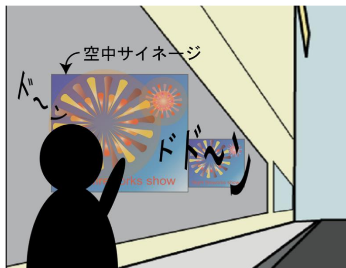
Fig.1-1. Digital signage that is formed by multi-modal aerial image. When you go through the signs, warmth via skin and sound can be also perceived from the aerial image position.
