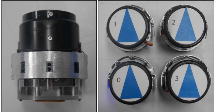
Figure 5.3: Installed distance sensors and markers
