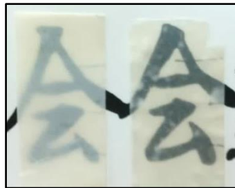
Figure 4.11: Transparency level of hot-pressed BC sheet (left) and BC/PVA sheet (right).
