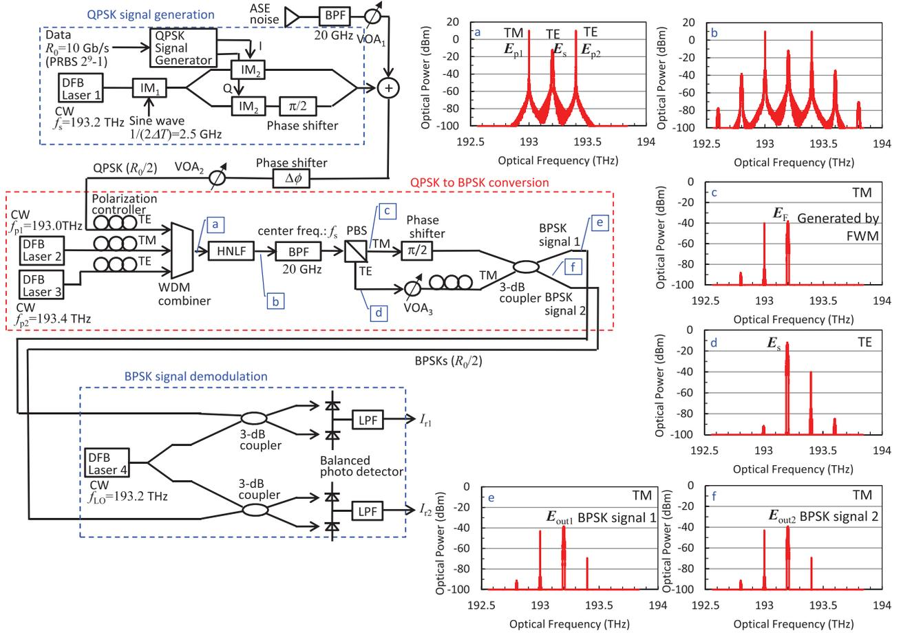
**Fig. 3** Setup used in numerical simulation. Optical spectra are shown as insets.
