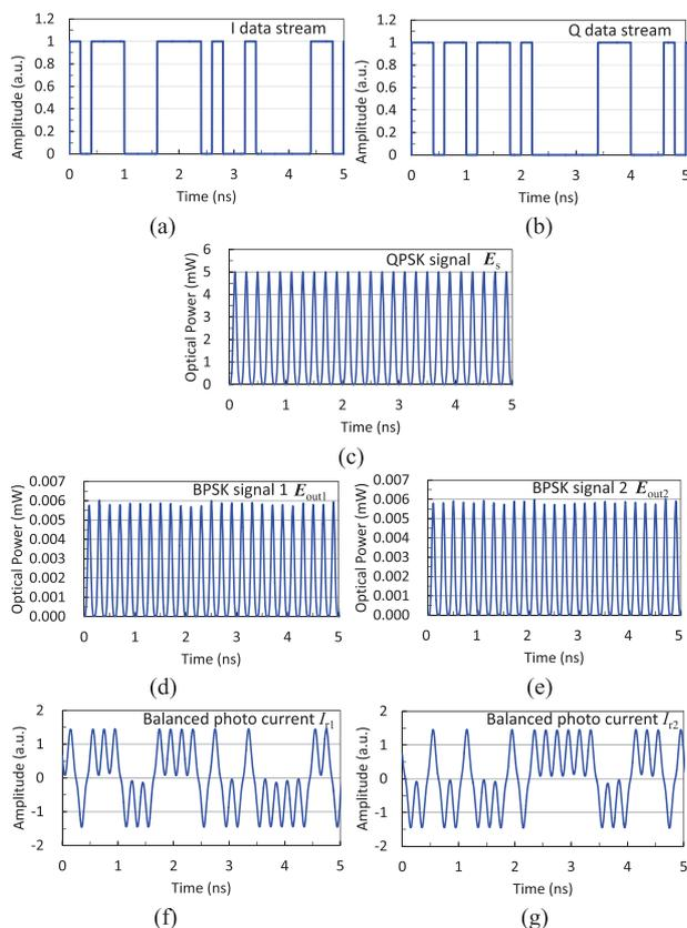
**Fig. 4** Optical waveform through format conversion by HNLFF; (a) NRZ  $I$  signal for QPSK modulation, (b) NRZ  $Q$  signal for QPSK modulation, (c) generated RZ QPSK signal, (d) converted BPSK signal 1, (e) converted BPSK signal 2, (f) balanced detected photo current  $I_{r1}$ , and (g) balanced detected photo current  $I_{r2}$ .
