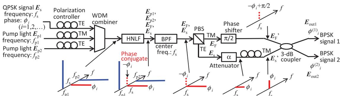
**Fig. 1** All-optical wavelength-shift-free modulation format converter from a QPSK stream to two BPSK tributaries using FWM in a HNLf.
