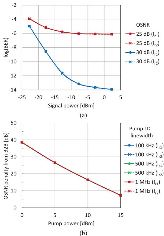
**Fig. 6** BER performance of the format conversion; (a) BER as a function of the signal power at the WDM combiner with pump power of 10 dBm, and (b) OSNR penalty from back-to-back result, where the linewidth of the pump lights is varied as a parameter.
