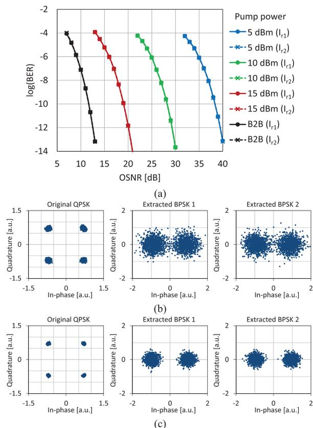
**Fig. 5** BER performance and constellation examples of the format conversion; (a) BER as a function of OSNR with pump power of 5 dBm, 10 dBm, and 15 dBm, and the signal power of 2.25 dBm at the WDM combiner, (b) constellation map of original QPSK signal and extracted two BPSK signals at pump power of 10 dBm and OSNR of 22 dB, and (c) 28 dB.
