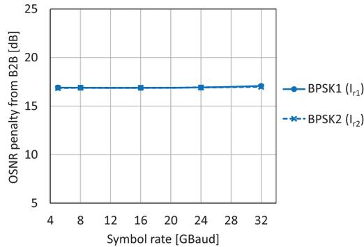
**Fig. 8** OSNR penalty from back-to-back result as a function of the symbol rate 5, 8, 16, 24, and 32 Gbaud.
