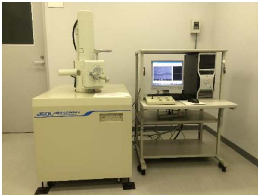
Figure 5.1 The fiber microstructure was measured by SEM
