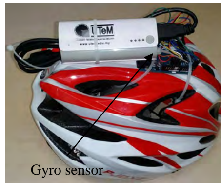
Figure 5.22: Installation of gyro sensor on the helmet
