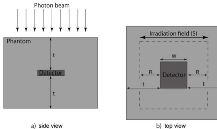
The detection region (10 mm×10 mm×2 mm) was **totally covered with** phantom. Here, size of irradiation field ( $S \times S$ ) was defined by  $S = R + 10 \text{ mm} + R$ , where **R** is **range** of secondary electron.
