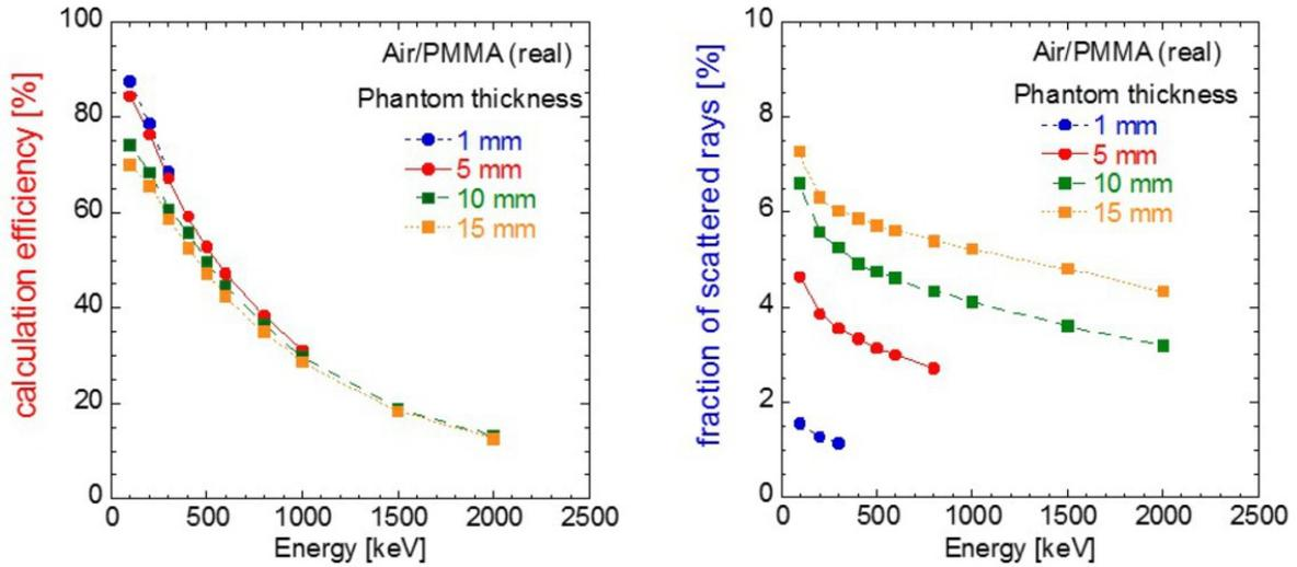
Fig. 9: Result of efficiency of Monte-Carlo simulation and fraction of scattered rays.
