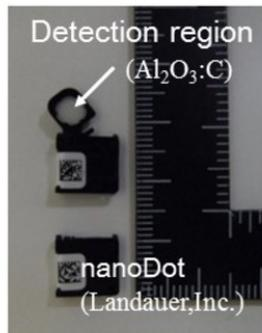
Small-type optically stimulated luminescence (OSL) dosimeter, called “**nanoDot**”, was recently made commercially available by Landauer Inc.
