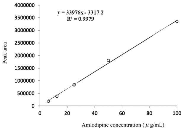
Figure 3. Calibration curve of amlodipine.
