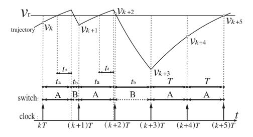
Figure 2: Behavior of the orbit with switching delay.
