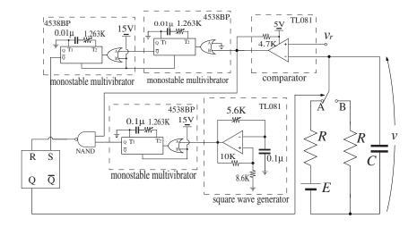
Figure 1: Circuit realization of chaotic switching system.
