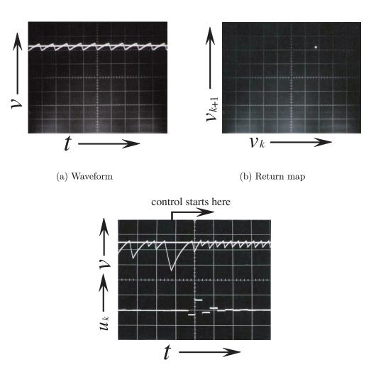
(c) Transient behavior of control waveform and control input
