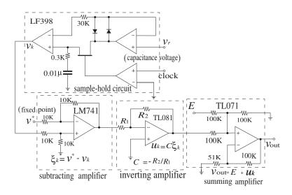
Figure 4: Block diagram of controller.
