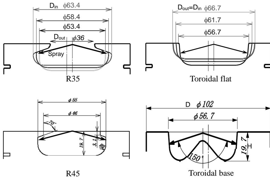
**Fig.3.** Piston configurations.
