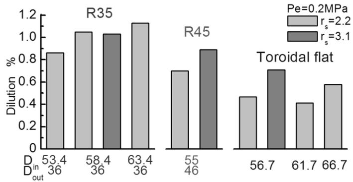
**Fig.5.** Comparison of fuel dilution in lubricating oil.
