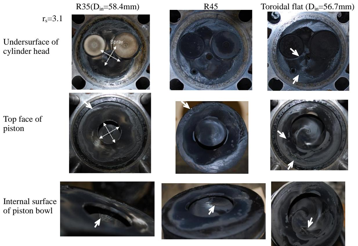
**Fig.6.** Deposit formation on the wall surface.
