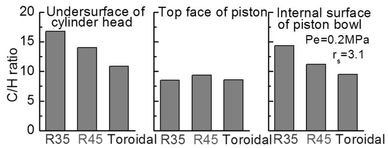
**Fig.8.** Elementary analysis (C/H ratio) of deposit.
