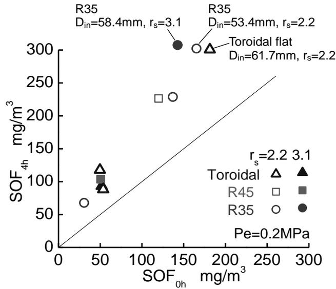
**Fig.13.** SOF emission before and after four hours continuous operation.
