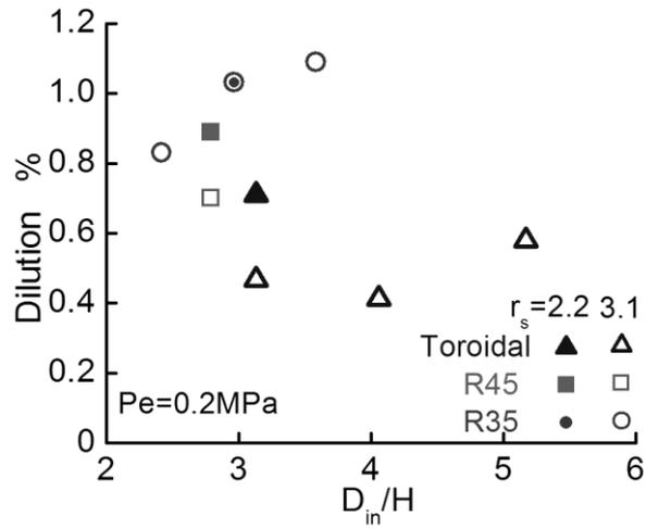
**Fig.10.** Relation between aspect ratio and fuel dilution in lubricating oil.
