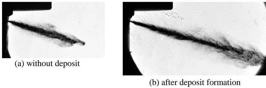
**Fig.14.** Change in spray characteristics before and after deposit formation in the nozzle hole [20]. (Injection pressure is 70MPa. Images are captured at 0.5ms aSOI under ambient condition of 298K and 1MPa.) (a) without deposit. (b) after deposit formation.
