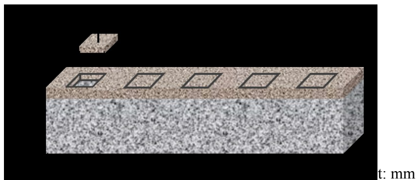
Fig. 7 Outline of the joint specimen for bond strength test of repair materials
