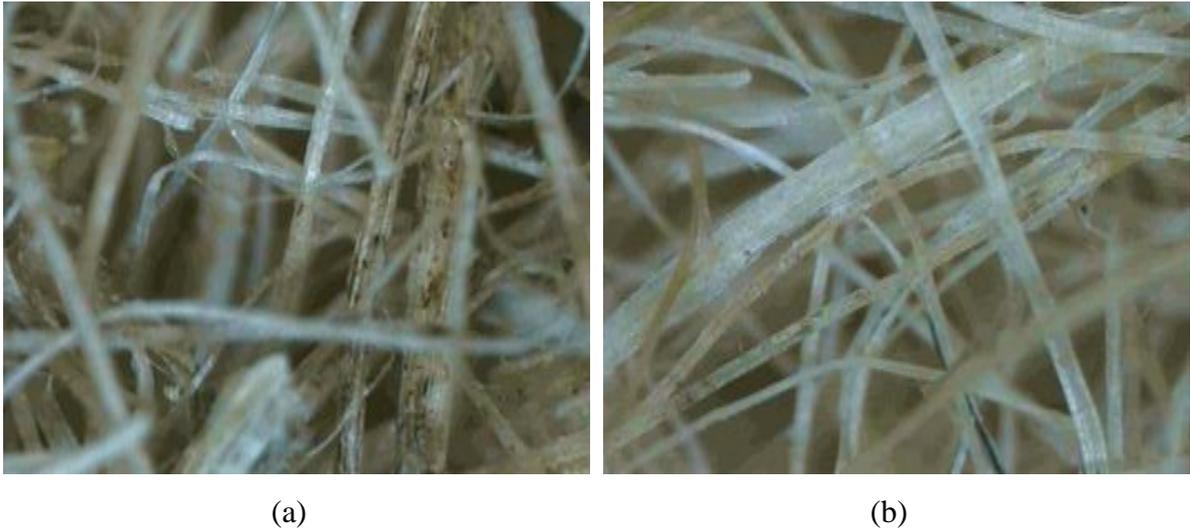
Figure 3.4: Non-woven kenaf fibres; a) KF before alkaline treated: corrupted and fungi, b) KF after alkaline treated: clean, shiny surfaces and free of impurities (10x Magnification).
