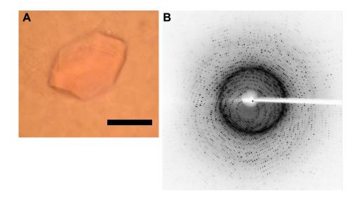
Fig. S1. A precipitant-free glucose isomerase crystal obtained by centrifugal concentration and typical diffraction spots of the crystal.
