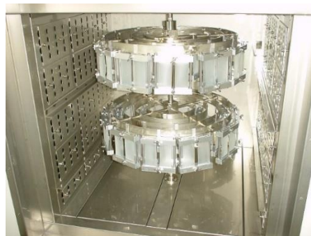
Fig 2.2 Heated situation in gear-type aging oven
