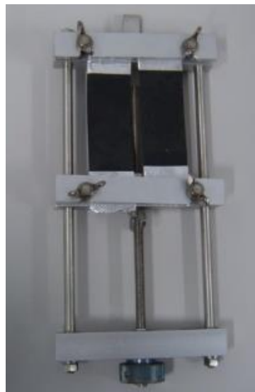
Fig 2.23 EPR tapes fitted in sample holder
