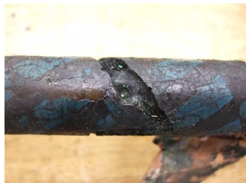
(b) Aspect of the breakdown point
