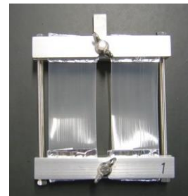
(b) XLPE sheet fitted in sample holder
