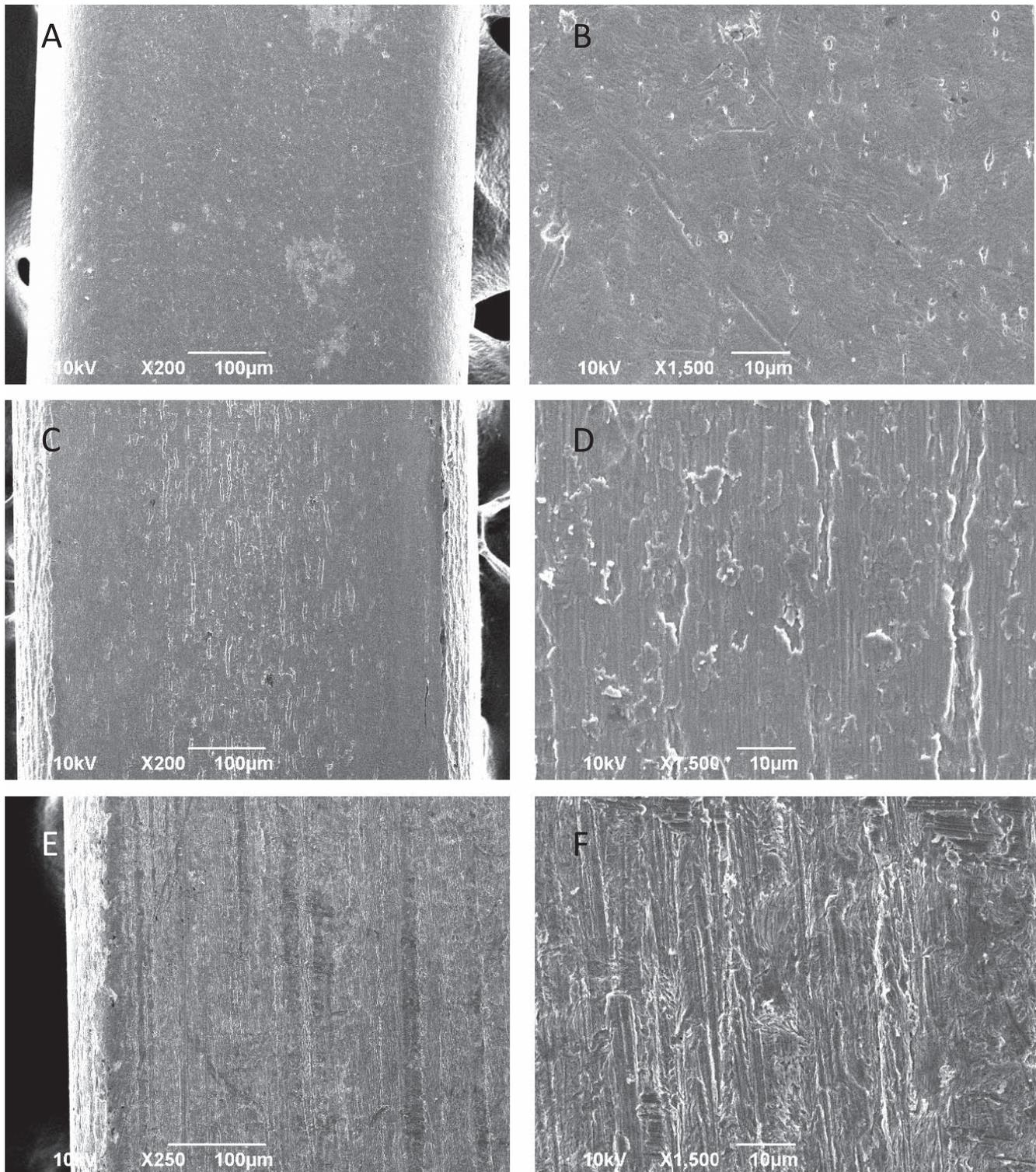
**Figure 4.** Scanning electron micrographs of orthodontic alloy wires. (A, B) Ti-Ni alloy wire, (C, D) Ti-Nb alloy wire, (E, F) Ti-Mo alloy wire. A, C, E: 250 $\times$  magnification; B, D, F: 1500 $\times$  magnification.
