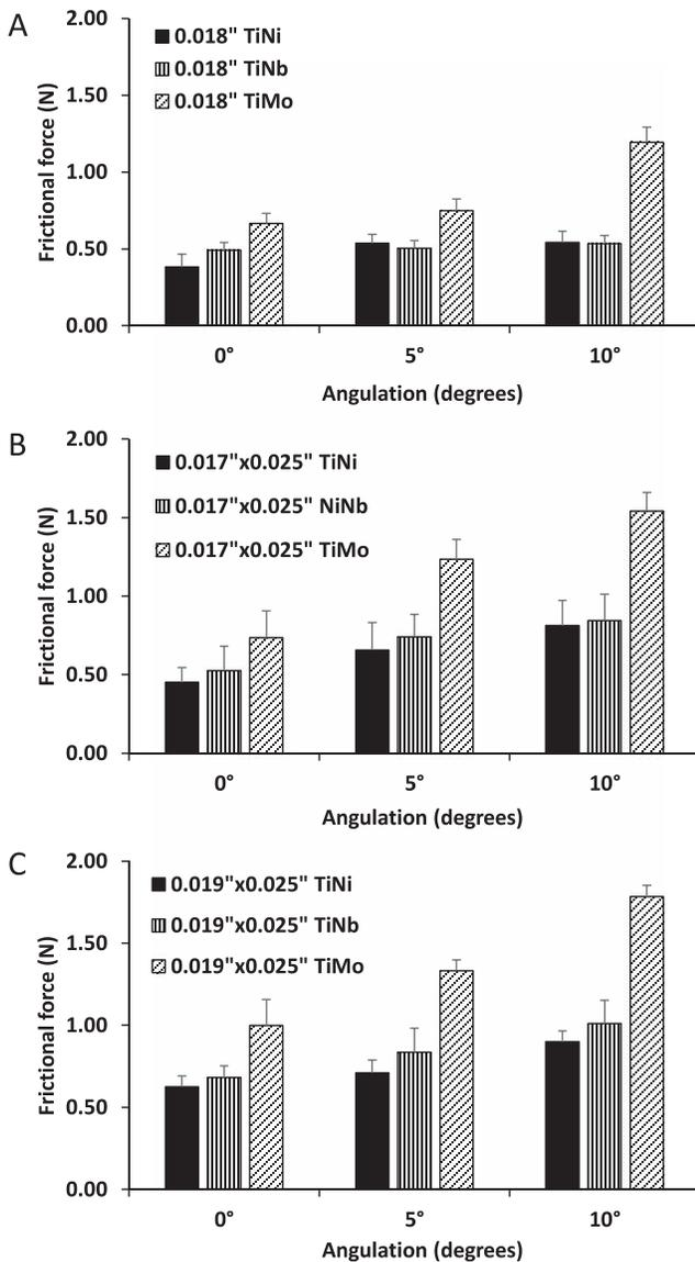
**Figure 3.** Frictional forces produced by orthodontic alloy wires in the 0.022-inch-slot bracket. (A) A 0.018-inch round wire, (B) 0.017 × 0.025-inch rectangular wire, (C) 0.019 × 0.025-inch rectangular wire (n = 15 per group).
