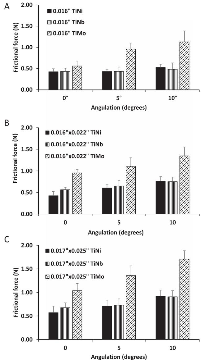
**Figure 2.** Frictional forces produced by orthodontic alloy wires in the 0.018-inch-slot bracket. (A) A 0.016-inch round wire, (B) 0.016 × 0.022-inch rectangular wire, (C) 0.017 × 0.025-inch rectangular wire (n = 15 per group).
