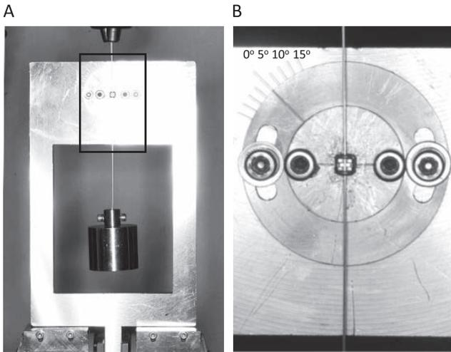
**Figure 1.** The testing machine, bracket-wire assembly, and force-measuring equipment. (A) Rotation fixture. (B) Inner aluminum block. (C) Outer aluminum block. (D) Anterior-posterior adjustable block. (E) Weight (150 g). (F) Horizontal adjustable joint. (G) Anterior-posterior adjusting handle.<sup>11</sup>
