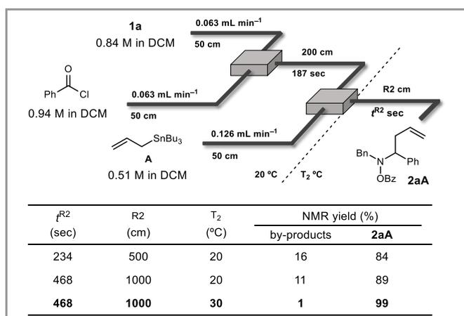
**Figure 3** Optimization of flow system conditions for the addition of **A** to **1a** via the formation of **Im(OBz)-1a**.
