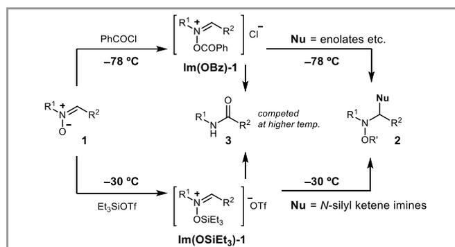
**Figure 1** Previous strategies for utilizing nitrones as electrophiles via their *N*-oxyiminium ion forms in batch system.<sup>4,6</sup>
