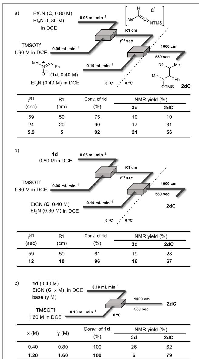
Figure 5 Optimization of flow system conditions for the addition of **C** to **1d** via the formation of **Im(OSiR<sub>3</sub>)-1d**.
