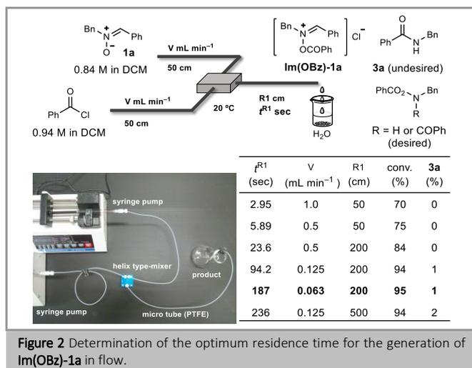
**Figure 2** Determination of the optimum residence time for the generation of **Im(OBz)-1a** in flow.
