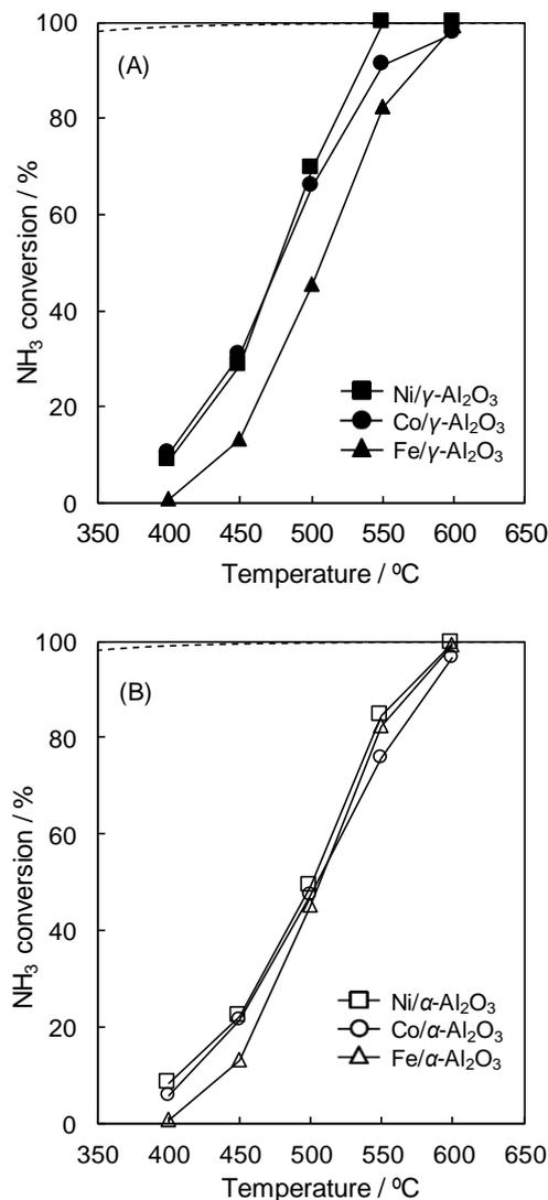
**Fig. 1** NH<sub>3</sub> conversion for NH<sub>3</sub> decomposition over (A)  $\gamma$ -Al<sub>2</sub>O<sub>3</sub> and (B)  $\alpha$ -Al<sub>2</sub>O<sub>3</sub> supported mono-metal catalysts: (square) Ni, (circle) Co, (triangle) Fe. Reaction conditions: 1.02% NH<sub>3</sub>/Ar balance; W/F: 2.45 kg-cat s L-NH<sub>3</sub><sup>-1</sup>; catalyst weight: 0.050 g. (dot-line) equilibrium NH<sub>3</sub> conversion.
