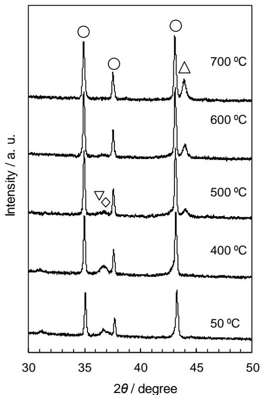
**Fig. 9** *In-situ* high temperature XRD patterns for the prepared Ni-Co/ $\alpha\text{-Al}_2\text{O}_3$  catalyst with the  $\text{Co}/(\text{Co}+\text{Ni})$  of 0.5. Symbols: (○)  $\alpha\text{-Al}_2\text{O}_3$ , (◇)  $\text{Co}_3\text{O}_4$ , (▽) NiO, (△) Ni or Co. Measurement atmosphere: 4%  $\text{H}_2/\text{Ar}$ .
