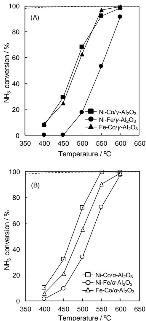
**Fig. 2** NH<sub>3</sub> conversion for NH<sub>3</sub> decomposition over (A)  $\gamma$ -Al<sub>2</sub>O<sub>3</sub> and (B)  $\alpha$ -Al<sub>2</sub>O<sub>3</sub> supported bi-metal catalysts: (square) Ni-Co, (circle) Ni-Fe, (triangle) Fe-Co. The molar ratio of both metals = 1:1. Reaction conditions: 1.02% NH<sub>3</sub>/Ar balance; W/F: 2.45 kg-cat s L-NH<sub>3</sub><sup>-1</sup>; catalyst weight: 0.050 g. (dot-line) equilibrium NH<sub>3</sub> conversion.
