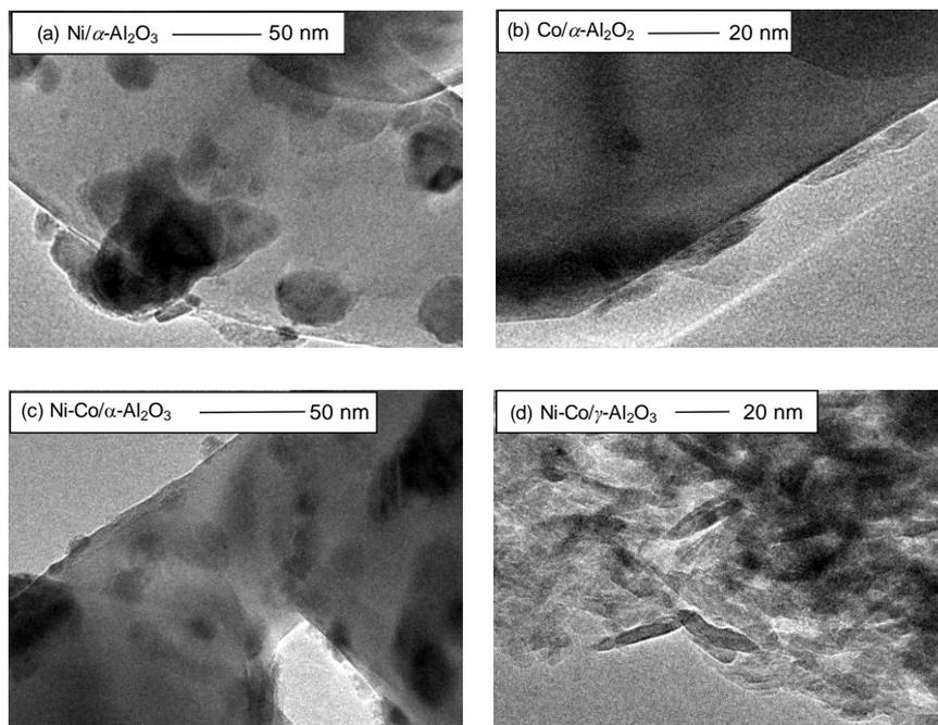
**Fig. 6** TEM images of the spent catalysts: (a) Ni/ $\alpha$ -Al<sub>2</sub>O<sub>3</sub>, (b) Co/ $\alpha$ -Al<sub>2</sub>O<sub>3</sub>, (c) Ni-Co/ $\alpha$ -Al<sub>2</sub>O<sub>3</sub>, (d) Ni-Co/ $\gamma$ -Al<sub>2</sub>O<sub>3</sub>.
