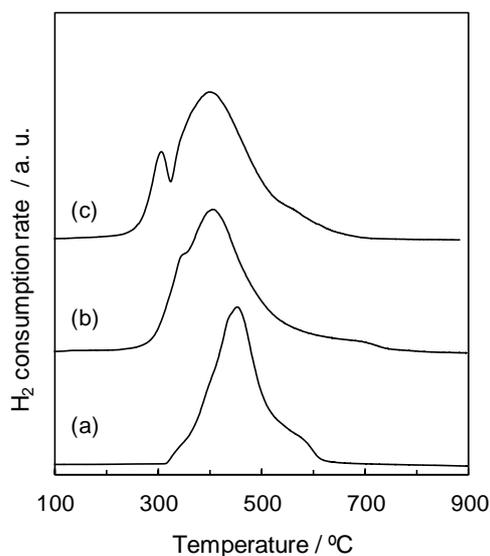
**Fig. 5** H<sub>2</sub>-TPR profiles of the prepared Ni and Co based catalysts: (a) Ni/ $\alpha$ -Al<sub>2</sub>O<sub>3</sub>, (b) Co/ $\alpha$ -Al<sub>2</sub>O<sub>3</sub>, (c) Ni-Co/ $\alpha$ -Al<sub>2</sub>O<sub>3</sub>.
