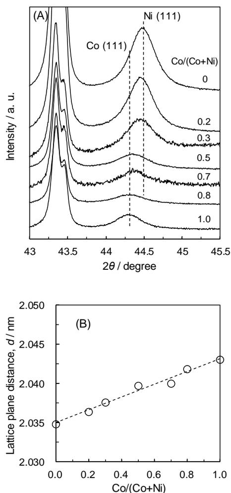
**Fig. 8** (A) XRD patterns and (B) relationship between  $\text{Co}/(\text{Co}+\text{Ni})$  and lattice plane distance for the spent Ni-Co/ $\alpha\text{-Al}_2\text{O}_3$  catalysts after  $\text{NH}_3$  decomposition tests.
