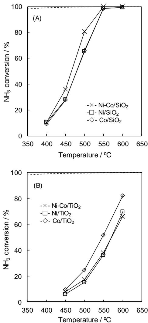
**Fig. 10** NH<sub>3</sub> conversion for NH<sub>3</sub> decomposition over (A) SiO<sub>2</sub> and (B) TiO<sub>2</sub> supported Ni and Co based catalysts. Reaction conditions: 1.02% NH<sub>3</sub>/Ar balance; W/F: 2.45 kg-cat s L-NH<sub>3</sub><sup>-1</sup>; catalyst weight: 0.050 g. (dot-line) equilibrium NH<sub>3</sub> conversion.
