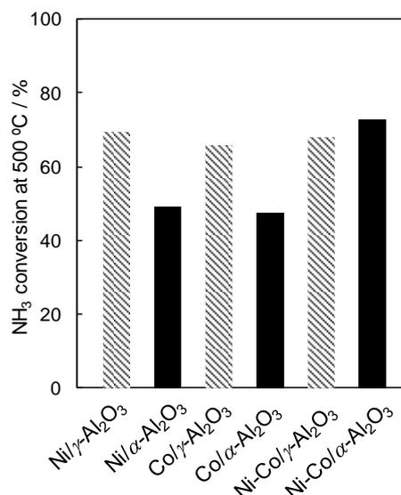
**Fig. 3** NH<sub>3</sub> conversion at 500 °C for Ni and Co based catalysts for NH<sub>3</sub> decomposition tests shown in Figs. 1 and 2.
