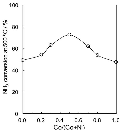
**Fig. 7** Effect of molar ratio of Co/(Co+Ni) on NH<sub>3</sub> conversion at 500 °C over Ni-Co/ $\alpha$ -Al<sub>2</sub>O<sub>3</sub> catalysts.
