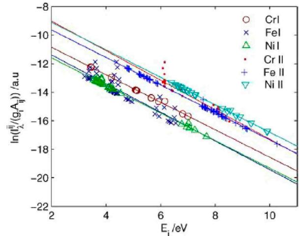
**Fig. 10.** Boltzmann plot corrected by the IRSAC for the iron-chromium-nickel alloy sample<sup>96)</sup> “Reprinted with permission from (L. X. Sun and H. B. Yu: Correction of self-absorption effect in calibration-free laser-induced breakdown spectroscopy by an internal reference method. *Talanta*. 2009; 79, 388–395. DOI:10.1016/j.talanta.2009.03.066). Copyright (2009) Elsevier”. (Online version in color.)
