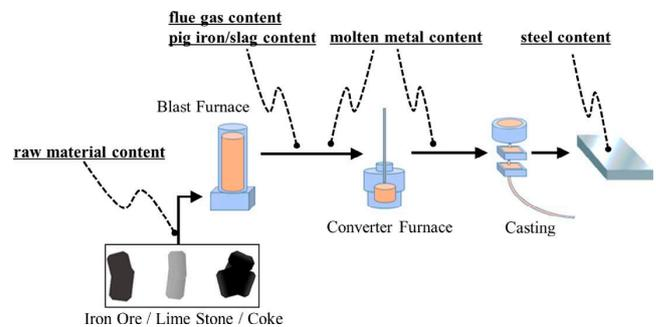
Fig. 5. Technical flow chart for the typical iron and steel making processes. (Online version in color.)
