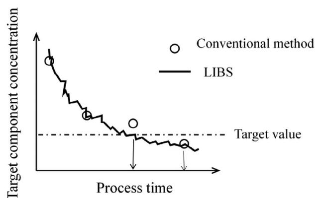
**Fig. 7.** Process control concept of target component concentration using a conventional method and LIBS technique.
