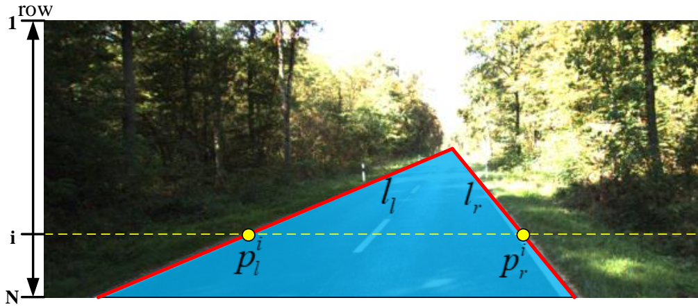
Figure 4.3: Road surface and boundary detection in the traffic image
