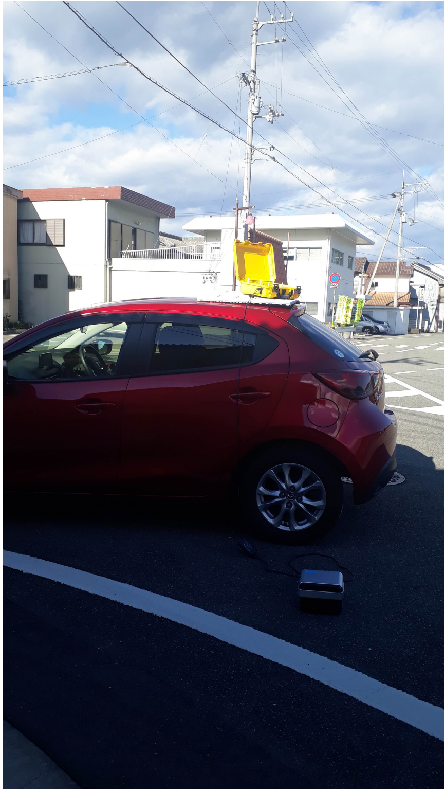
Figure. 4.13: Spare AP Implementation of Disaster Field Experiment
