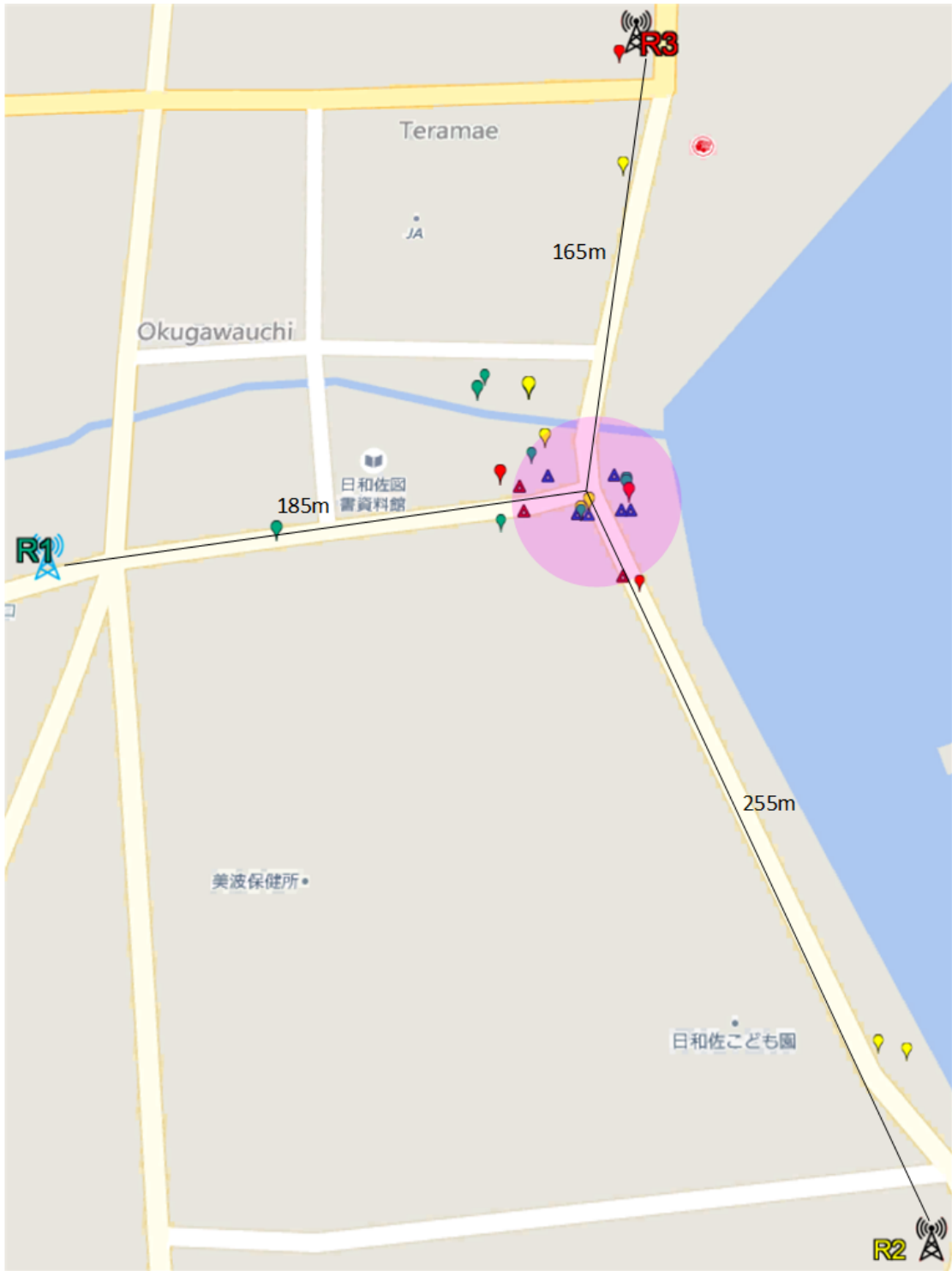
Figure. 4.11: Routers and Spare AP Locations
