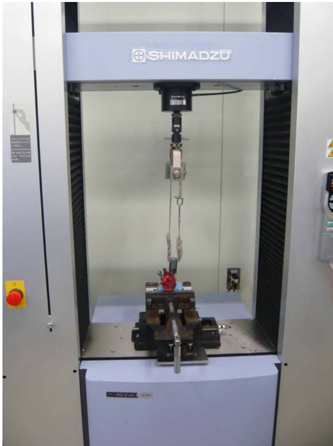
Figure 5 Screw pullout testing; the testing special adaptors were made to fit securely around the screw head.
