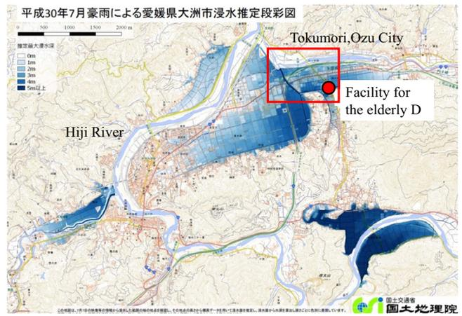
**Fig. 11.** Locations of flooded area near Hiji River and facility D (Created by modifying a gradient tints diagram of inundation around Hiji River due to the heavy rain in July 2018 created by the Geospatial Information Authority of Japan).
