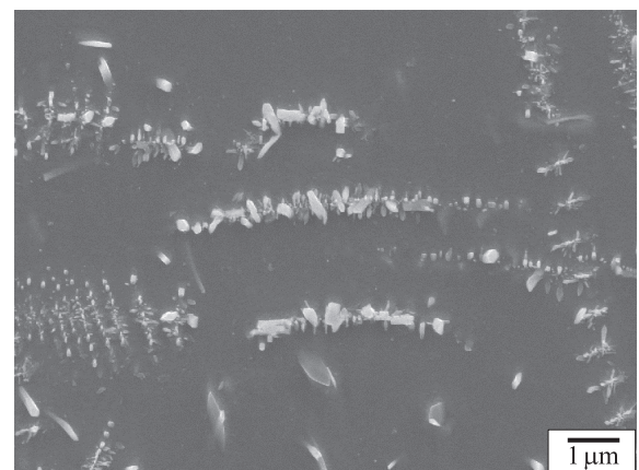
Fig. 11 SEM SEI of HR6W creep-interrupted at 973 K/120 MPa for 2872 h.
