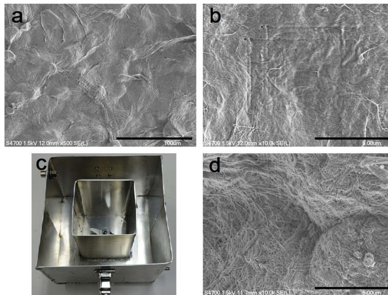
Fig. 1. Scanning electron micrographs of: (a) sudachi nanofiber, scale bar 100  $\mu\text{m}$ ; (b) sudachi nanofiber, scale bar 5  $\mu\text{m}$ ; (c) modified blender bottle; (d) commercial nanofiber Celish, scale bar 5  $\mu\text{m}$ .
