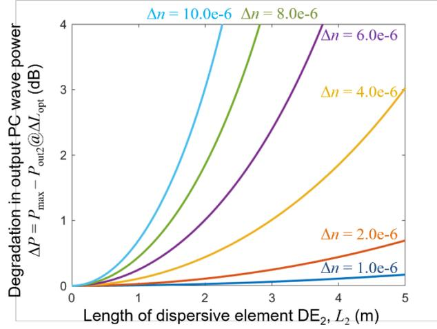
**Fig. 4** Degradation  $\Delta P$  in output PC wave power as function of  $DE_2$  length,  $L_2$ . Shift  $\Delta n$  in refractive index varies from  $1.0e-6$  to  $10.0e-6$
