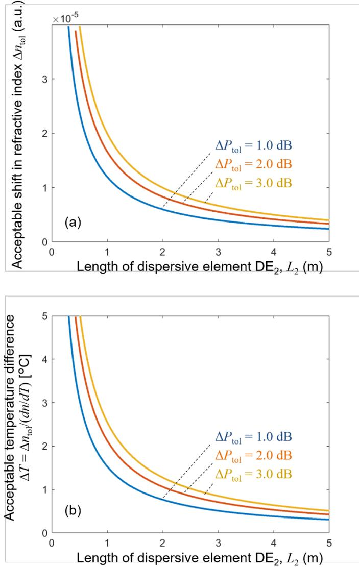
**Fig. 5** (a) Acceptable shift in refractive index and (b) temperature difference as a function of  $\text{DE}_2$  length,  $L_2$
