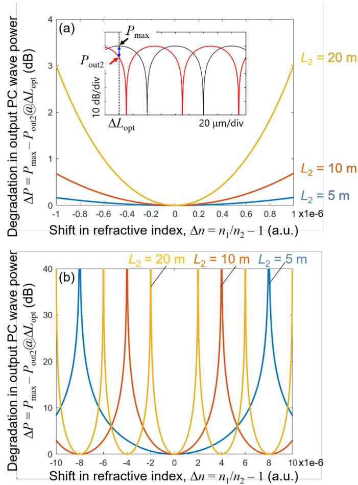
**Fig. 3** Degradation  $\Delta P$  in output PC wave power as function of shift  $\Delta n$  in refractive index. Blue, orange, and yellow lines represent the cases  $L_2 = 5, 10, 20$  m, respectively. (a)  $\Delta n$  ranges from  $-1.0\text{e-}6$  to  $+1.0\text{e-}6$ ; (b)  $\Delta n$  ranges from  $-10.0\text{e-}6$  to  $+10.0\text{e-}6$
