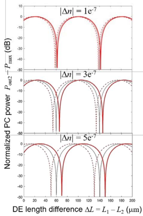
**Fig. 2** Normalized output PC wave power  $P_{\text{out}2} - P_{\text{max}}$  as a function of difference in DE lengths,  $\Delta L$ . Black solid lines indicate  $\Delta n = 0$  and dashed and bold solid red lines indicate  $+\Delta n$  and  $-\Delta n$
