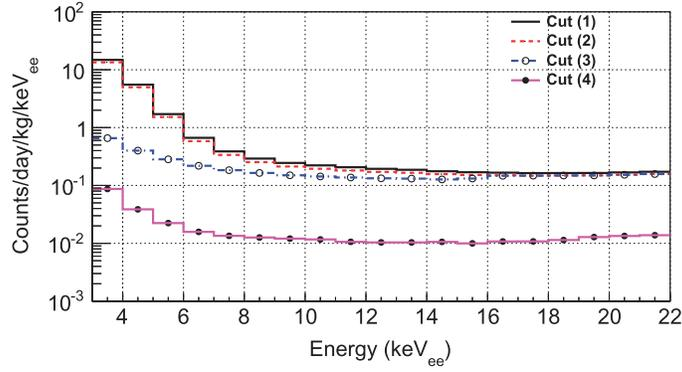
**Fig. 4.** Energy spectra of the observed data after each reduction step. The histogram with the black solid line shows the events after cut (1), the red dotted line shows the events after cut (2), the blue dash-dotted line represents the events after cut (3), and the magenta solid line with filled circle shows the events after cut (4), which is the final sample.
