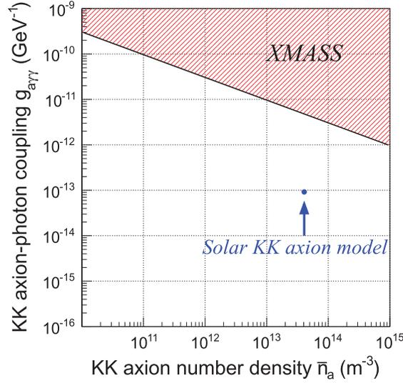
**Fig. 6.** The obtained 90% CL excluded region from this work is shown by the black solid slope and the red hatched area. The model assumed in this study based on Ref. [8] is indicated by the blue point.
