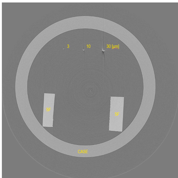
Fig. 2. Tomographic slice in the transversal direction of the micro-wire phantom consisting of 3, 10, and 30 \mu\text{m} diameter wires.
