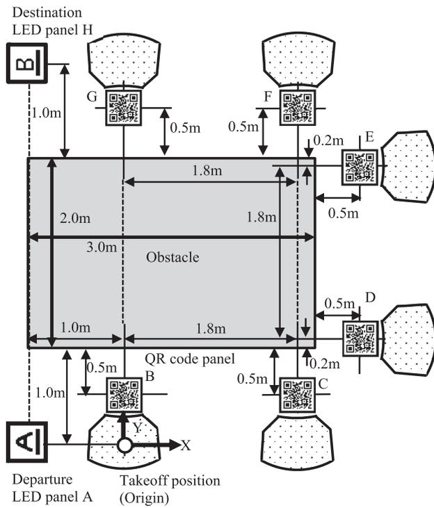
**Fig. 11.** Layout of LED and QR code panels for flight experiments.
