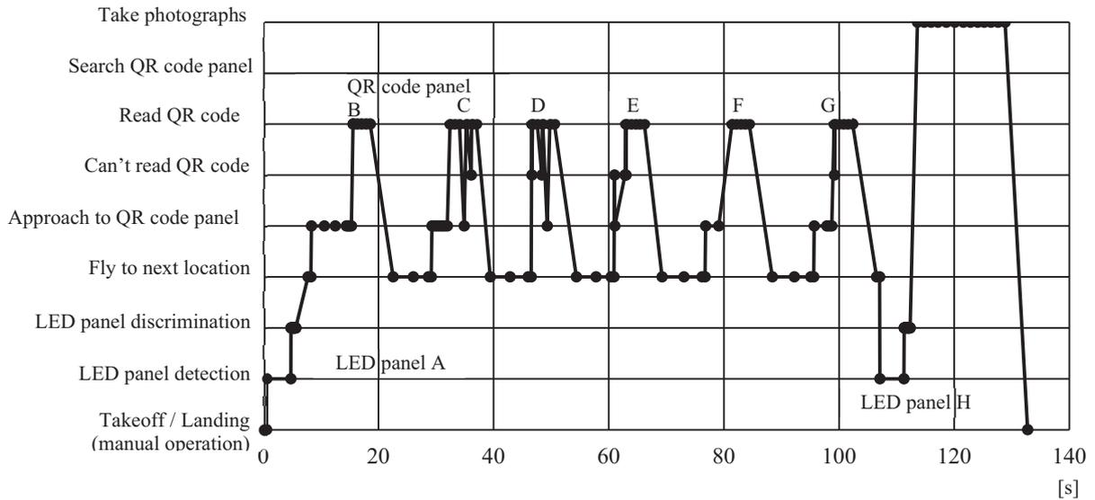
**Fig. 17.** Timing chart of UAV state.
