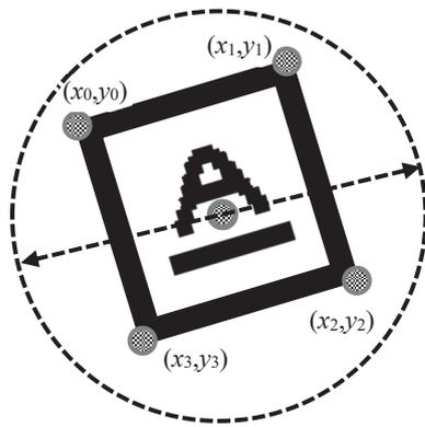
**Fig. 5.** Black frame extraction on LED panel image and obtain four corner points.
