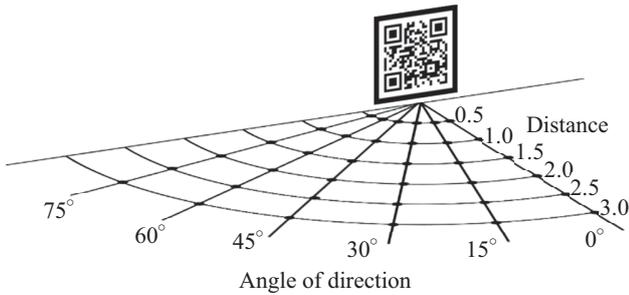
**Fig. 10.** Arrangement of camera for QR code panel.
