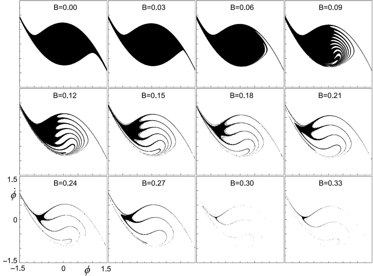
**Fig. 5.** Fractal metamorphoses of basin boundary in initial value plane with  $\kappa = 0.04455$  and  $\omega = 0.905$  (This figure duplicates Fig. 9 in the literature [14]), but at higher resolution).
