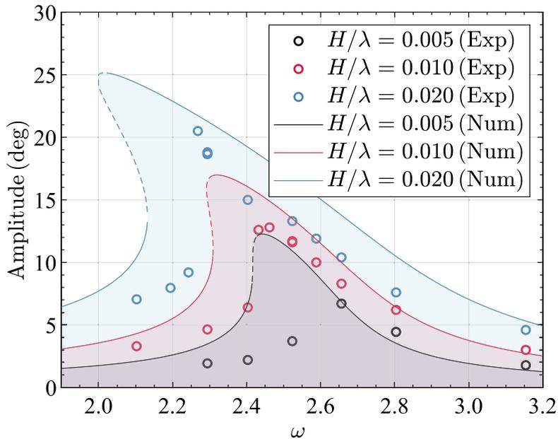
**Fig. 12.** Response amplitude of the model ship CEHIPAR2792. A part of the data is included in [36]. The lines show the results of the averaging method.
