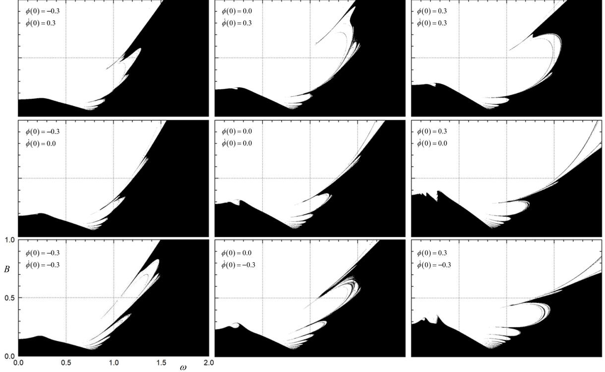
**Fig. 7.** Fractal metamorphoses of basin boundary in control space with  $\kappa = 0.04455$  for different sets of initial values  $\phi(0)$  and  $\dot{\phi}(0)$  (The center figure ( $\phi(0) = 0.0$  and  $\dot{\phi}(0) = 0.0$ ) duplicates Fig. 12 in the literature [14], but at high resolution).
