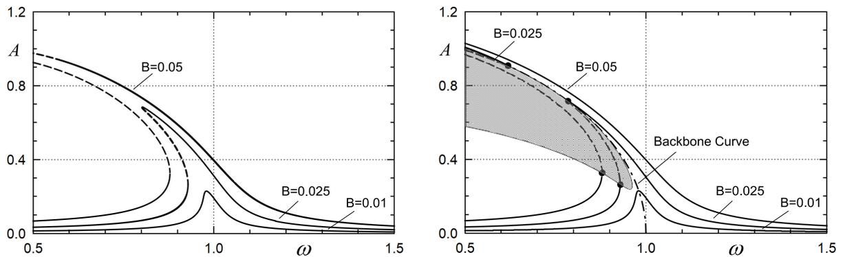
**Fig. 10.** Response amplitude of the primary motion with  $c_1 = 1$ ,  $c_3 = 1$ ,  $\kappa = 0.04455$  and  $B_0 = 0.0$ . The left panel represents the numerical solutions, and the right panel shows the analytical solutions. The solid and dashed lines indicate the stable and unstable regions, respectively. (This figure duplicates Fig. 1 in the literature [24]).
