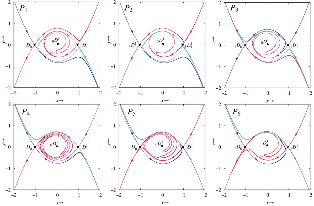
**Fig. 22.** Stable and unstable manifolds of the system (8) with the parameters of  $P_1$ – $P_6$ . This figure duplicates Fig. 5 in the literature [43] and the variables  $x$  and  $y$  here are equivalent to the variables  $\phi$  and  $\dot{\phi}$  in this manuscript, respectively.
