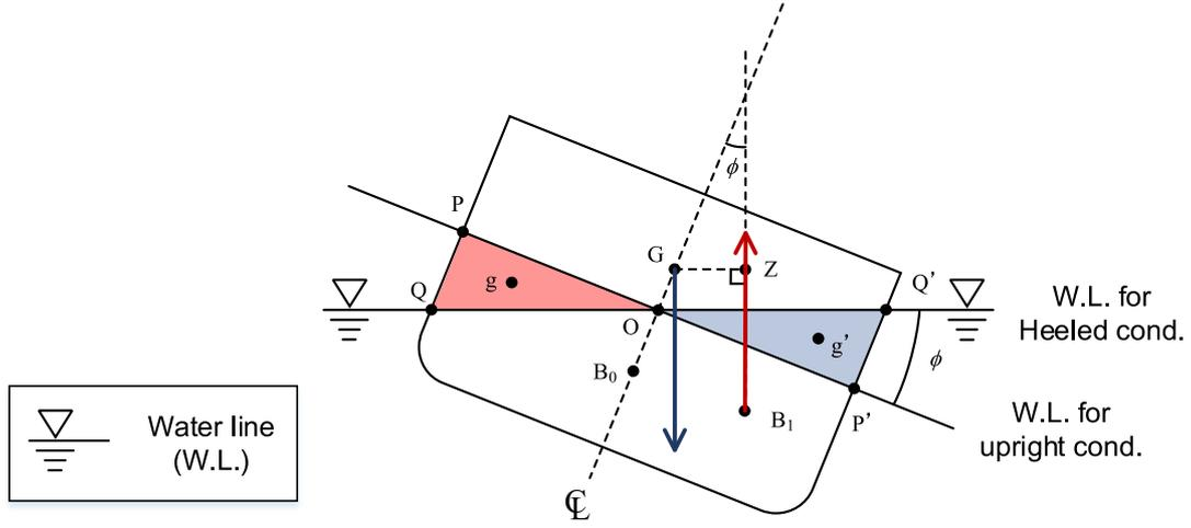
Fig. 1. Restoring moment for a wall-sided vessel.
