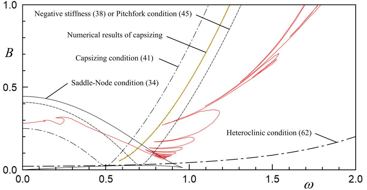
**Fig. 19.** Capsizing boundary and bifurcation sets with  $c_1 = 1$ ,  $c_3 = 1$ . Red line indicates the capsizing boundary for  $\phi = 0$  and  $\dot{\phi} = 0$  shown in Fig. 7. The part of the plots is included in [24].
