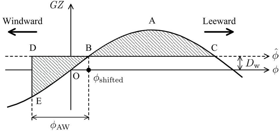
Fig. 4. Schematic of energy balance.
