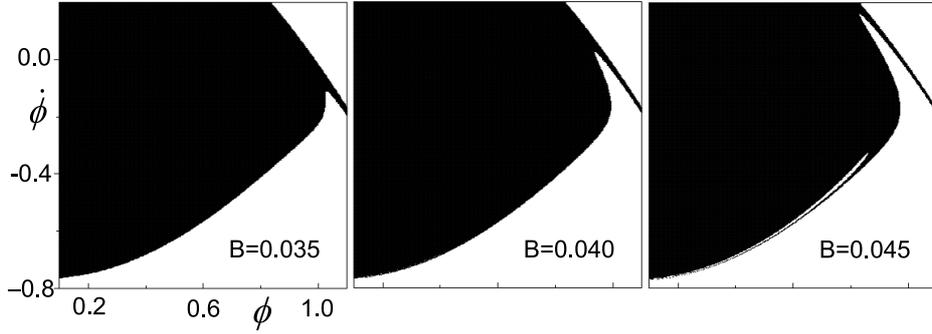
**Fig. 17.** Fractal metamorphoses of basin boundary in initial-value plane with  $\kappa = 0.04455$ . The threshold is calculated as  $B = 0.03830$  from Eq. (62).
