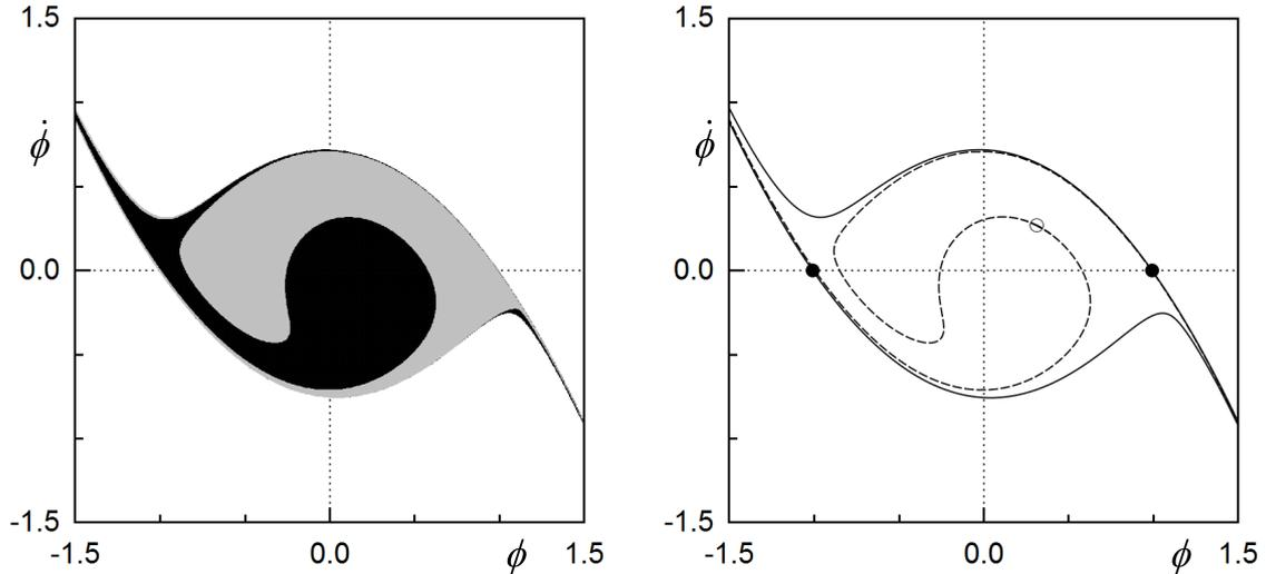
**Fig. 11.** Coexistence of the two solutions with  $c_1 = 1$ ,  $c_3 = 1$ ,  $B = 0.025$ ,  $\kappa = 0.04455$ ,  $\omega = 0.905$ . Black and gray regions show that with the initial conditions, the solution converges to a periodic attractor (fixed point, represented by the white points).
