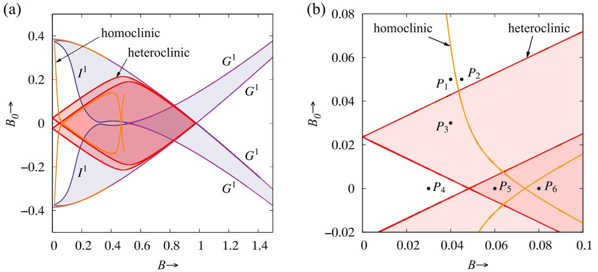
**Fig. 21.** Bifurcation sets of the system (8) with  $\kappa = 0.5$ ,  $c_1 = 1$ ,  $c_3 = 1$  and  $\omega = 1.0$  (this figure duplicates Fig. 1 in the literature [43]).  $G^1$  and  $I^1$  are saddle-node and period-doubling bifurcation sets, respectively.
