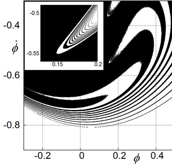
**Fig. 6.** Fractal magnification of metamorphoses of basin boundary in initial value plane with  $\kappa = 0.04455$ ,  $\omega = 0.905$  and  $B = 0.09$  (This figure duplicates Fig. 10 in the literature [14]), but at higher resolution).
