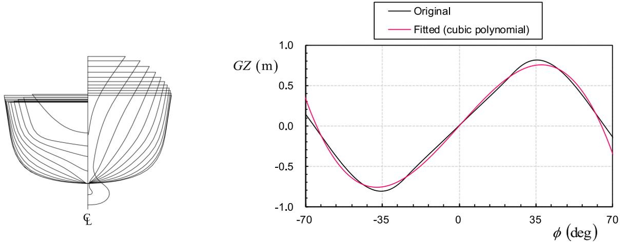
**Fig. 8.** Body plan of DTMB5415 hull form and its  $GZ$  curve. Here, cubic polynomial expression ( $c_1\phi - c_3\phi^3$ ) is also plotted.
