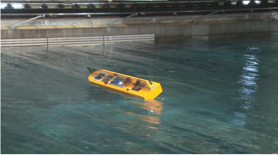
**Fig. 13.** Photo of the experiment for the model ship CEHIPAR2792 in the rectangular tank of the National Research Institute of Fisheries Engineering (NRIFE). Waves were generated by a wave maker located at the end of the tank (right side of this photo).
