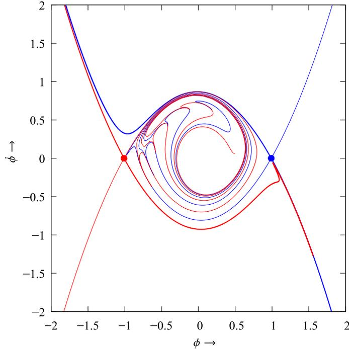
**Fig. 18.** Heteroclinic tangency with  $\kappa = 0.04455$  and  $B = 0.03830$  from Eq. (62). The blue and red curves are the manifolds for the blue and red saddles, respectively; thicker curves are the stable manifolds and thinner are the unstable ones.
