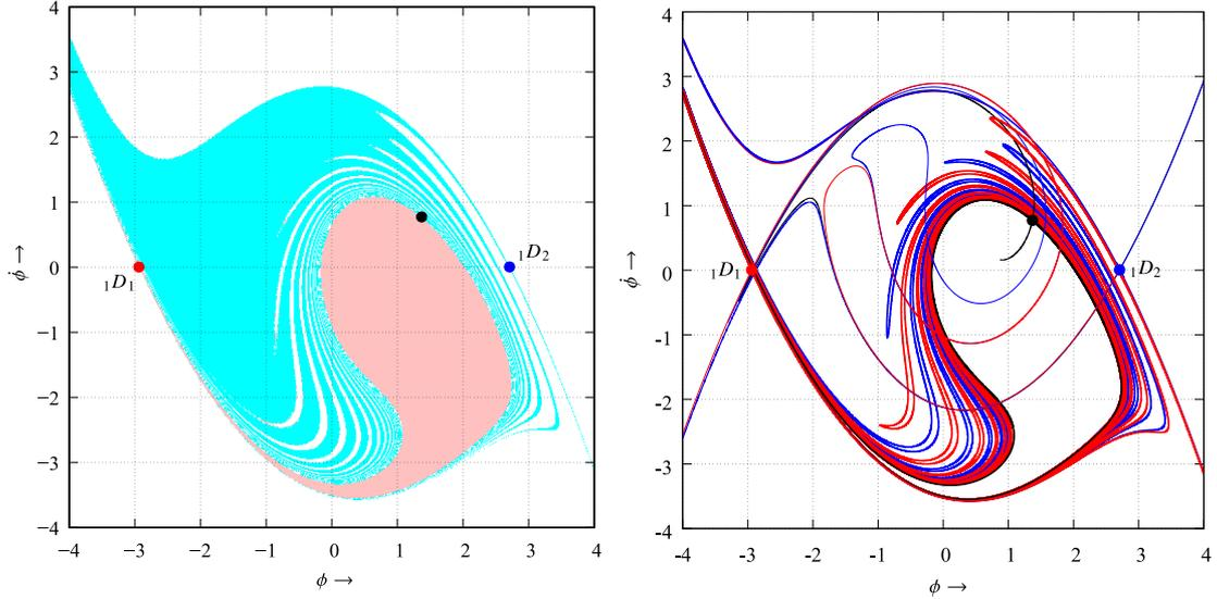
**Fig. 20.** Left panel: Fractal metamorphoses of basin boundary in the initial-value plane with  $\kappa = 0.17$ ,  $c_1 = 2$ ,  $c_3 = 0.25$ ,  $B_0 = 0$ ,  $B = 0.6$ , and  $\omega = 1.1$  (This figure duplicates Fig. 12 in the literature [10]), but at a higher resolution. Right panel: stable and unstable manifolds of two saddles,  ${}_1D_1$  and  ${}_1D_2$ , which are the red and blue points, respectively. Bolder curves are the stable manifolds and thinner curves are the unstable manifolds.
