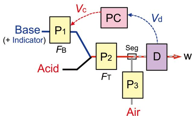
Fig. 1 Flow system for flow titration by flow ratiometry coupled with an air segmentation approach.  $P_1$ – $P_3$ , peristaltic pumps; Seg, segmenter; D, UV/Vis detector; PC, laptop computer with A/D-D/A converter; w, waste;  $F_B$ , flow rate of base solution;  $F_T$ , total flow rate of merged solution;  $V_c$ , control signal;  $V_d$ , detector output signal.
