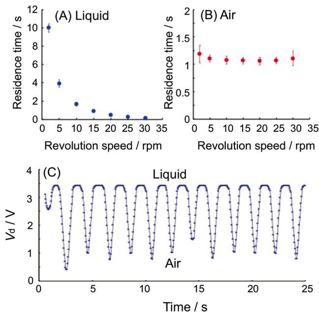
Fig. 3 Effect of the revolution speed of  $P_3$  on the residence time of  $0.05 \text{ mmol dm}^{-3}$  Erythrosine B segment (A) and on that of air bubble (B) in optical window. (C) Analytical signals at a  $P_3$  revolution speed of 15 rpm. Sampling frequency was 20 Hz.
