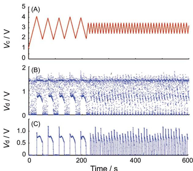
Fig. 4 Typical flow signals. (A) Control voltage,  $V_c$ . (B) Raw detector output voltage,  $V_d$ . (C) Software-based deaerated and smoothed  $V_d$ . Titrand,  $0.1 \text{ mol dm}^{-3}$  HCl; titrant,  $0.1 \text{ mol dm}^{-3}$  NaOH containing  $0.047 \text{ mmol dm}^{-3}$  Bromothymol Blue. Sampling frequency was 20 Hz.
