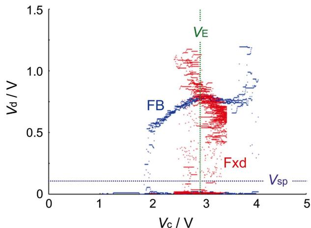
Fig. 5 Titration curve for the data given in Fig. 5. FB, data obtained in feedback-based mode; Fxd, data obtained in fixed triangular wave-controlled mode;  $V_E$ , controller output voltage that gives equivalence composition at the confluence point;  $V_{sp}$ ,  $V_d$  corresponding to the equivalence point.
