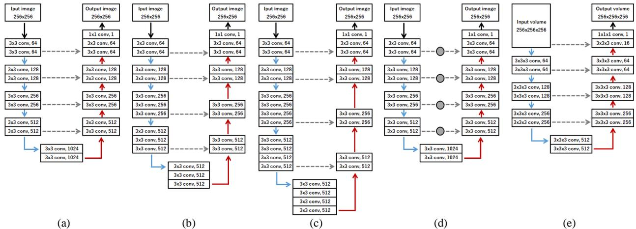
Fig. 2. 2D and 3D U-Net architectures. (a) 2D U-Net, (b) 2D U-Net with pretrained VGG-16 encoder, (c) 2D U-Net with pretrained VGG-19 encoder, (d) 2D attention U-Net, (e) 3D U-Net. Blue, red, and gray lines mean max pooling, transposed convolution, and copy. Black line means input or output. Gray circle means attention gate [17].
