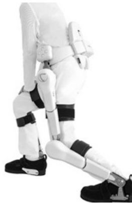
Fig. 1.6: Power assist device HAL (Cyberdyne Co.)
