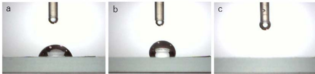
Figure 4. The shapes of the water drops applied to each sample. (a) Control; (b) Acid; (c) Alkali group.
