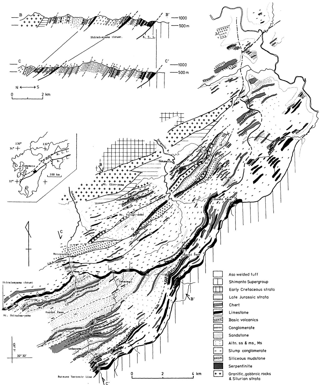
Fig. 3. Geological map and cross sections of the Gokase area. Arrows in the cross sections show the facings of the strata.
