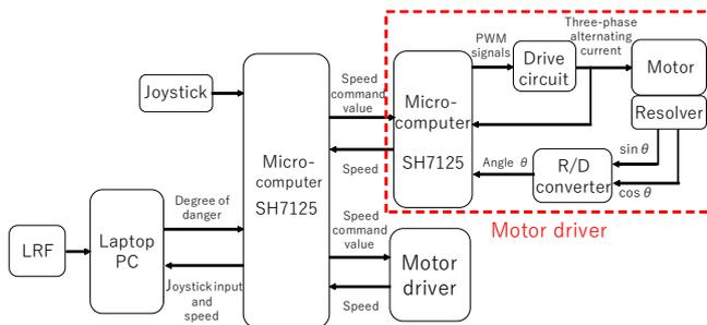
Figure 2: Hardware configuration of electric wheelchair
