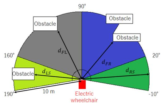
Figure 4: Definition of scanning area of LRF
