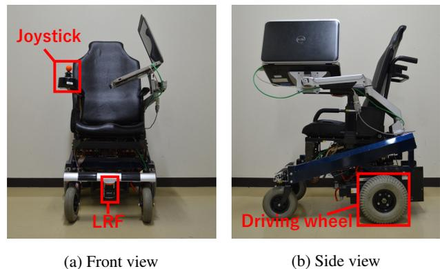
Figure 1: Appearance of developed electric wheelchair
