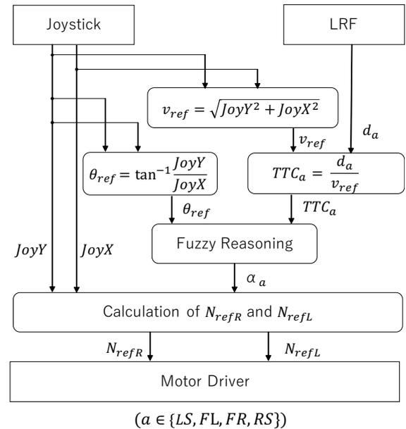
Figure 3: Safe driving support system
