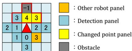
Figure 7: Point placement for detection area after two actions
