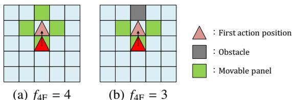
Figure 8: Degree of freedom of moving for robot
