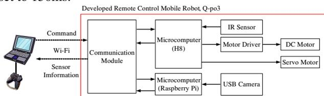
Figure 2: Hardware configuration
