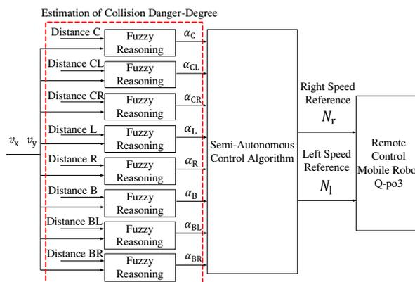
Figure 4: Configuration of proposed control system
