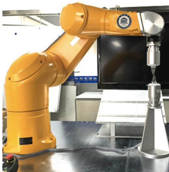
Figure 5. Novel robot system for orthodontic archwire bending [38].
