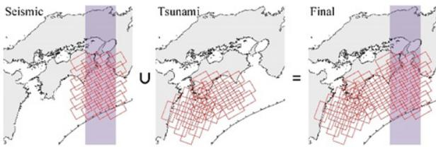
**Fig. 7.** Narrowing down fault models using seismic and tsunami data.
