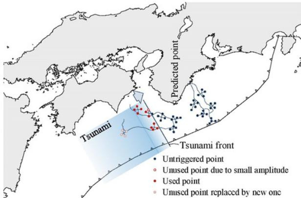
**Fig. 8.** Dynamic selection of DONET stations. Closed and open red circles respectively indicate triggered DONET stations and stations removed from among those triggered.
