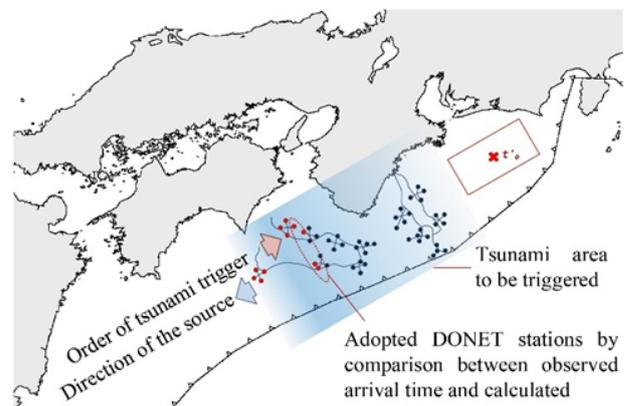
**Fig. 6.** Selection of fault models based on the tsunami trigger pattern at DONET stations.
