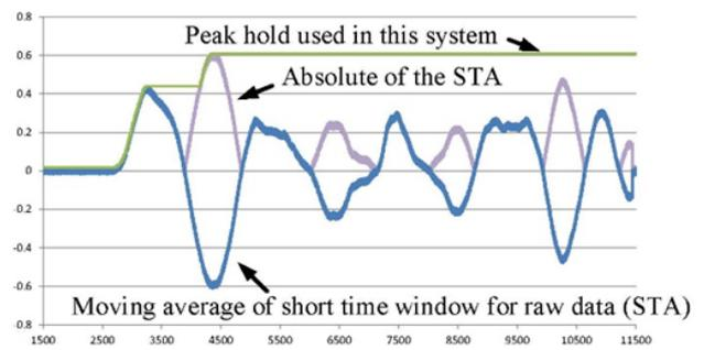
**Fig. 3.** Data processing for data input. Blue and purple lines represent the original waveform and absolute values, respectively. The peak-hold waveform of the purple graph is used as the input (green line) of the system.
