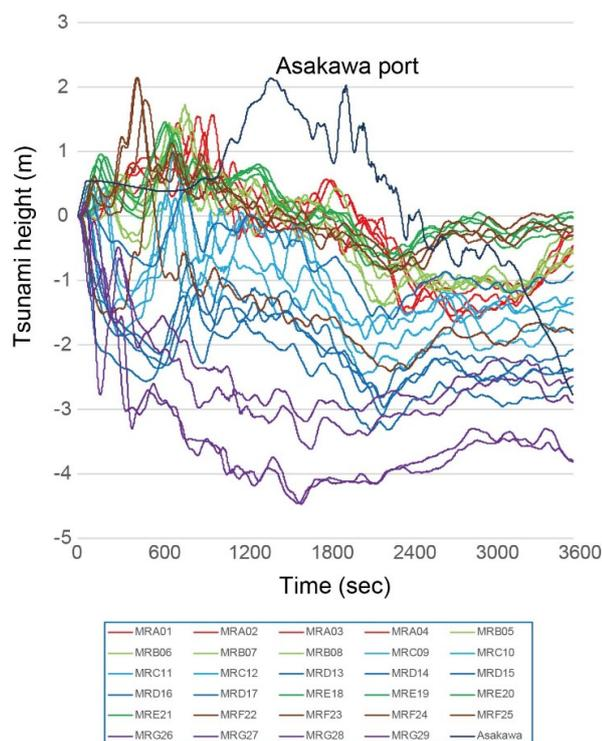
**Fig. 10.** Calculated waveforms of pressure gauges of DONET2 stations and tsunami height at Asakawa port, the town of Kaiyo, Tokushima, using Model Case 5 proposed by the Japan Cabinet Office. Stations indicated by the same color are connected to a single node.
