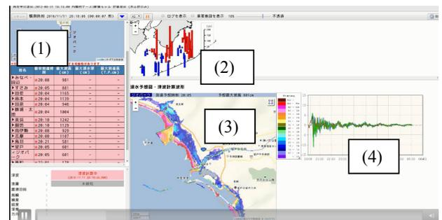
**Fig. 4.** Example of the tsunami prediction system display. The table of predicted tsunami arrival time and maximum tsunami height (1), real-time DONET data (2), inundation map (3), and calculated tsunami waveform at the predicted point using extracted fault models (4) are displayed in a single window.
