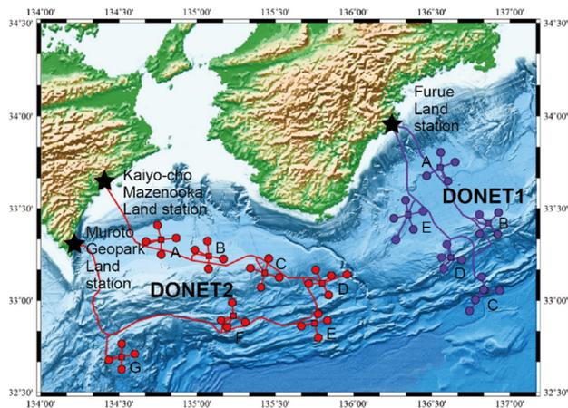
**Fig. 1.** Map of DONET installation. Observatories of DONET1 and DONET2 are indicated by purple and red circles, respectively. Stars are land stations. Squares with alphabet letters indicate nodes (branching apparatuses).
