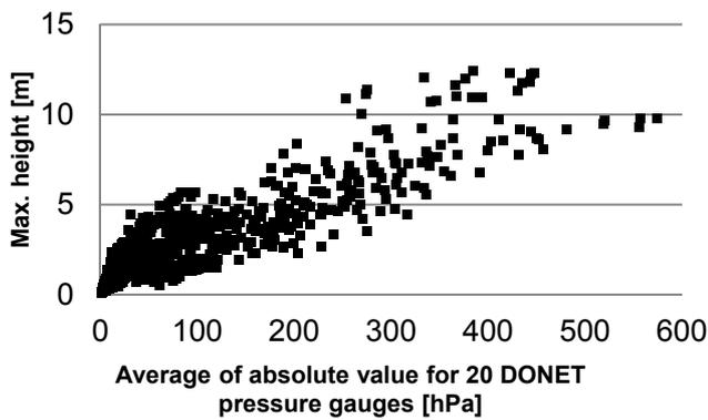
**Fig. 2.** Example of correlation diagram between DONET input data and maximum tsunami height at coastal target point.
