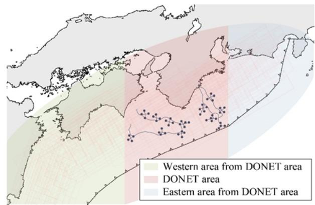
**Fig. 5.** Identification of the source region. The system identifies the source region by comparing the travel times of P-waves between DONET stations and narrows down the fault models.
