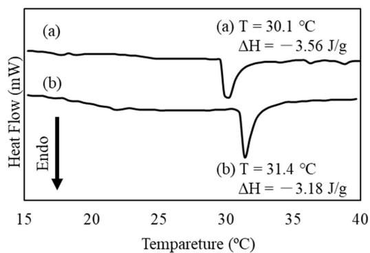
**Figure 5.** The analysis data of thermosensitive properties of PTMCM-MOE3OM and PTMCE-MOE4OM. DSC curves of PTMCM-MOE3OM (a) and PTMCE-MOE4OM (b) solutions in water at 0.5 mg/mL during second heating (heating rate 2.0 °C/min).
