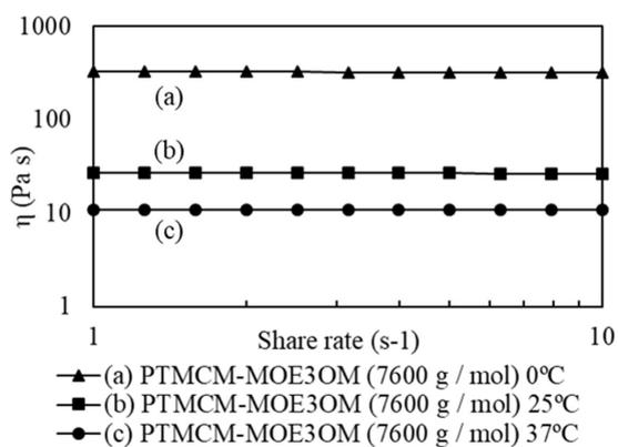
**Figure 4.** The viscosity character of PTMCM-MOE3OM vs sheare rate at 0 °C (a), 25 °C (b), and 37 °C (c).
