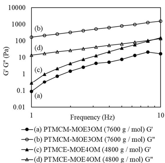
**Figure 1.** The analysis data of rheometer measurement of PTMCM-MOE3OM and PTMCE-MOE4OM. The viscoelastic character vs frequency storage modulus (a) and loss modulus (b) of PTMCM-MOE3OM and storage modulus (c) and loss modulus (d) of PTMCE-MOE4OM at 25 °C.
