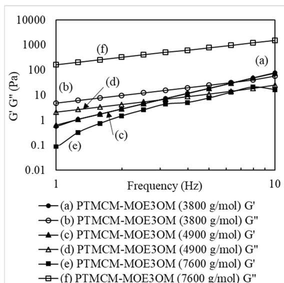
**Figure 2.** The viscoelastic character of PTMCM-MOE3OM vs frequency in each molecular weight. (a) Storage modulus of 3800 g/mol, (b) loss modulus of 3800 g/mol, (c) storage modulus of 4900 g/mol, (d) loss modulus of 4900 g/mol, (e) storage modulus of 7600 g/mol, and (f) loss modulus of 7600 g/mol.
