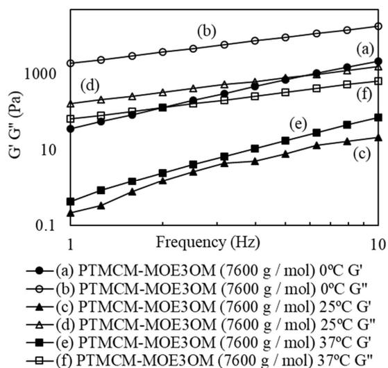
**Figure 3.** The viscoelastic character of PTMCM-MOE3OM vs frequency in each temperature. (a) Storage modulus at 0 °C, (b) loss modulus at 0 °C, (c) storage modulus at 25 °C, (d) loss modulus at 25 °C, (e) storage modulus at 37 °C, and (f) loss modulus at 37 °C.
