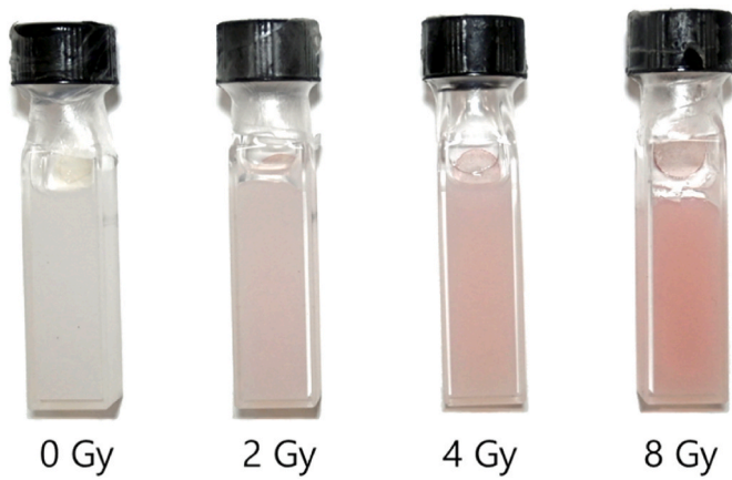
Fig. 1. A photograph of PAISiN samples; from the left, unirradiated one and those in few minutes after irradiation with X-rays (160 kV, 6.3 mA) at 8 Gy, 4 Gy, and 2 Gy, respectively.
