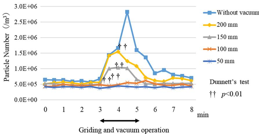
FIGURE 2 Typical time course of changes in the amount of particulate matter (silicone point; PMNs measuring 1.0 µm in diameter [d]; distance: 200 mm, angle: 90°).
