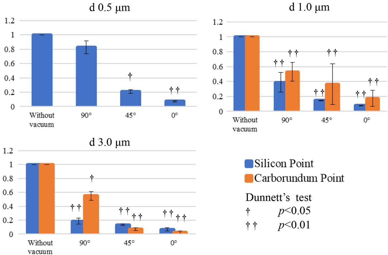
FIGURE 4 Reduction ratios: Influence of the angle between the grinding surface and extraoral vacuum on the maximum amount of particulate matter.
