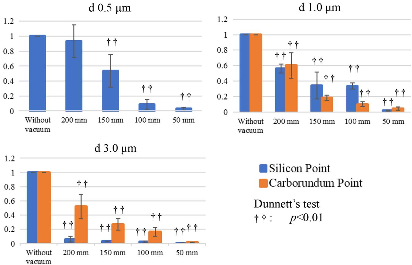
FIGURE 3 Reduction ratios: Influence of the distance between the grinding surface and extraoral vacuum on the maximum amount of particulate matter.
