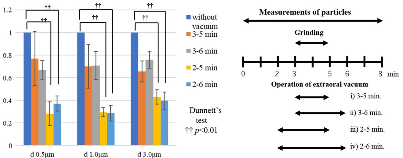
FIGURE 5 Reduction ratios: Influence of the operation time of the extraoral vacuum on the maximum amount of particulate matter: (silicone point; PMNs with the following diameters [d]: 0.5, 1.0, and 3.0 μm; distance: 200 mm, angle: 90°).
