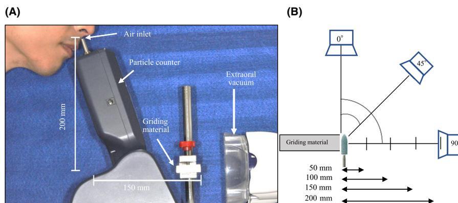
**FIGURE 1** Measurement conditions. (A) Positional relationship of the grinding material, air inlet of the particle counter, and extraoral vacuum. (B) Setup conditions for the distance and angle between the grinding material and the extraoral vacuum.
