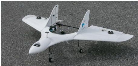
Fig. 2. First prototype of a tilt-rotor UAV (wingspan: 2.2 m).
