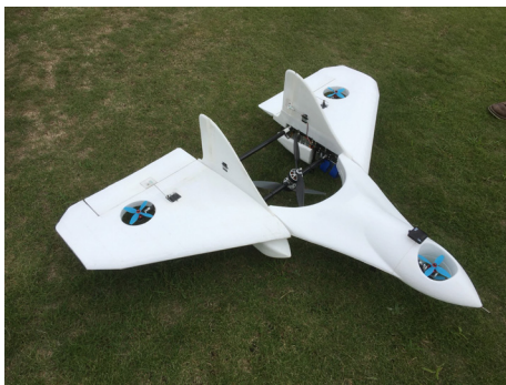
Fig. 3. Second prototype of a tilt-rotor UAV (wingspan: 1.43 m).
